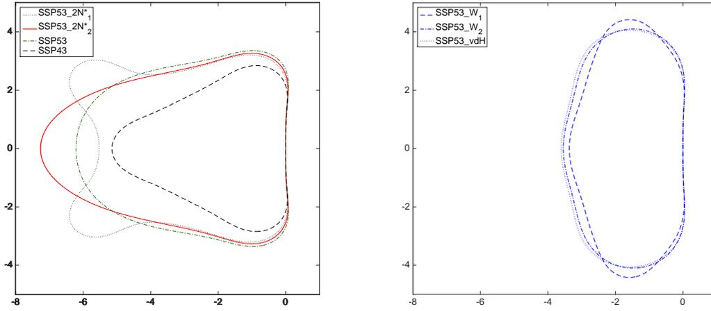
Figure 1: Stability regions for schemes SSP53\_2N<sub>1</sub><sup>\*</sup> (50), SSP53\_2N<sub>2</sub><sup>\*</sup> (53), SSP53 and SSP43 (left). Stability regions for schemes SSP53\_W<sub>1</sub>, SSP53\_W<sub>2</sub> and SSP53\_vdH (right).
