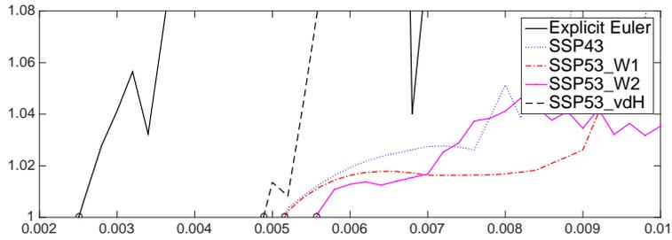
Figure 4: Ratio  $\mu(\Delta t)$  for the forward Euler method and other  $2N$  low-storage Runge-Kutta methods: SSP43 (23), SSP53\_W<sub>1</sub> (62), SSP53\_W<sub>2</sub> (63) and SSP53\_vdH (64).
