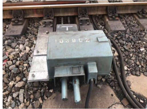
Fig. 3. Railway point machine
