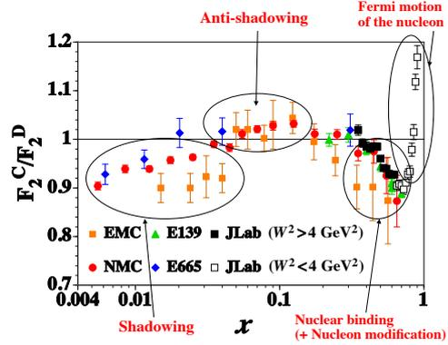
Figure 4: Nuclear modifications in  $F_2^C/F_2^D$ .
