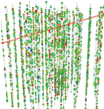
**Figure 7.** Simulated signal event of a horizontal magnetic monopole with speed  $0.01 c$ . The color, from red to blue, indicates the time evolution of the event. The total time of the event is 48 ms. The size of the spheres scales with the amount of light detected by each DOM. The original track of the particle is shown in red.
