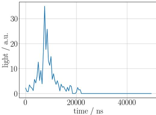
**Figure 5.** Spatially compressed light curve of a simulated magnetic monopole event. All light recorded by all DOMs is included and shown as a function of time.
