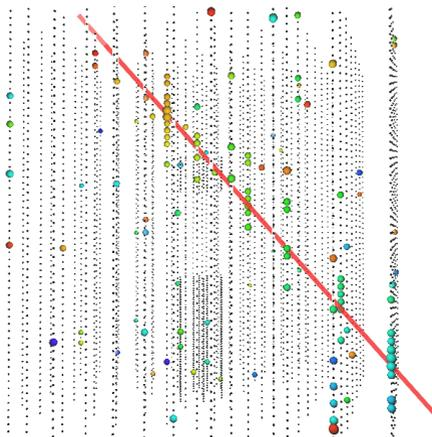
**Figure 4.** Simulated signal event of a magnetic monopole with speed  $0.3c$  moving from the top of the detector to the bottom (down going). The color, from red to blue, indicates the time evolution of the event. The total duration of the event is  $30\text{ }\mu\text{s}$ . The size of the spheres scales with the amount of light detected by each DOM. The original track of the particle was included in red. The hits far away from the track are noise hits.
