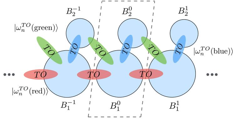
Figure 11: Metasurface and the periodic singular plasmons. The dotted lines represent the unit cell of the metasurface. The red, blue, green coloured arrays of ellipses represent the periodic singular plasmons basis  $|\omega_n^{TO}(red)\rangle$ ,  $|\omega_n^{TO}(blue)\rangle$ ,  $|\omega_n^{TO}(green)\rangle$ , respectively
