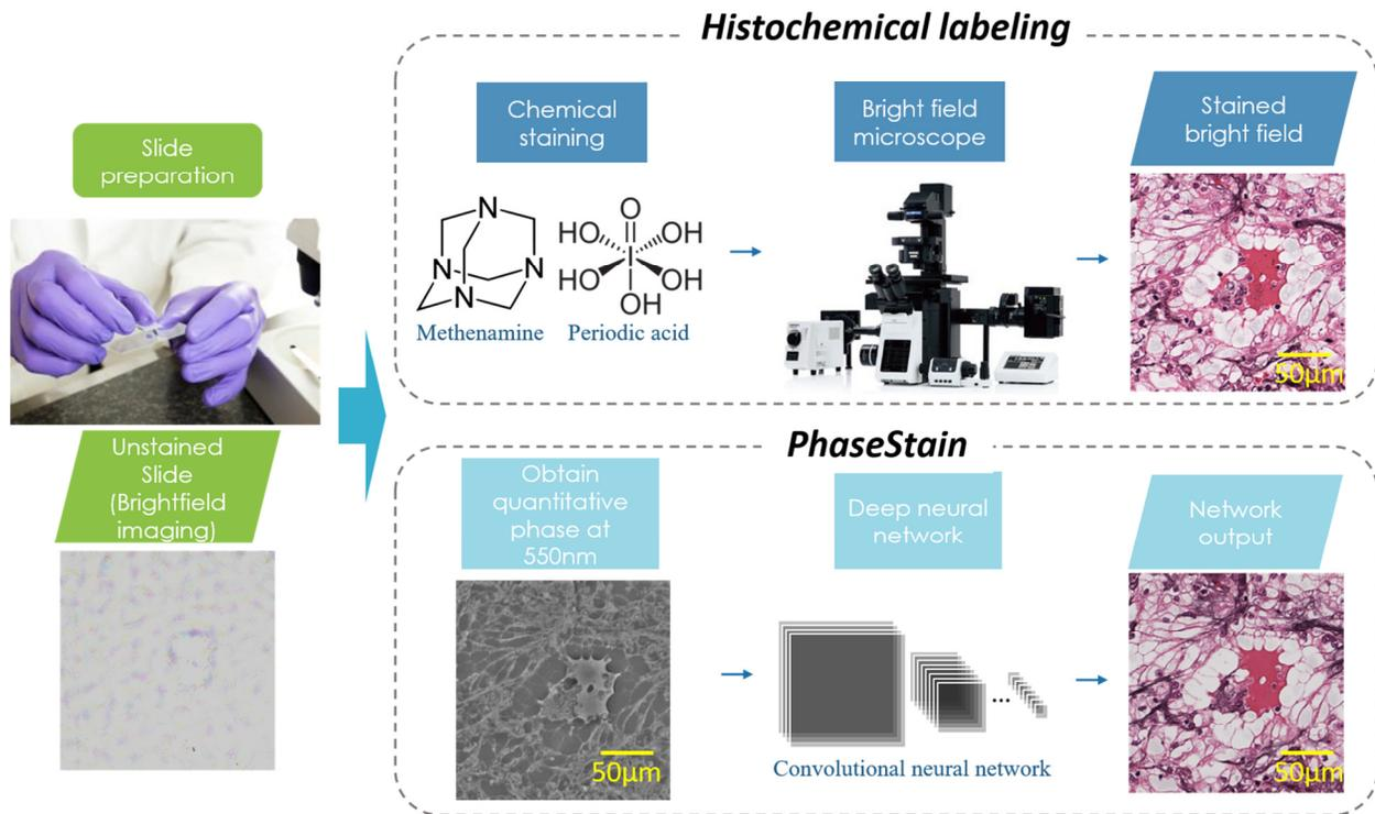
**Fig. 1.** PhaseStain workflow: Quantitative phase image of a label-free specimen is virtually stained by a deep neural network, bypassing the standard histochemical staining procedure that is used as part of clinical pathology.
