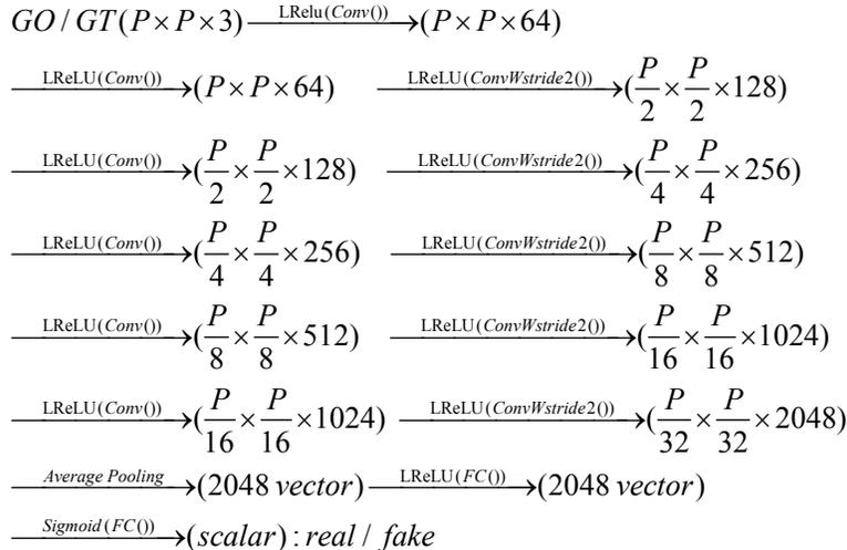
**Table 1.** The GAN architecture. LReLU: Leaky ReLU, Conv: convolutional layer with a stride of 1, FC: fully-connected layer, ConvWstride2: convolutional layer with stride 2, GO: generated output, GT: ground truth image.
