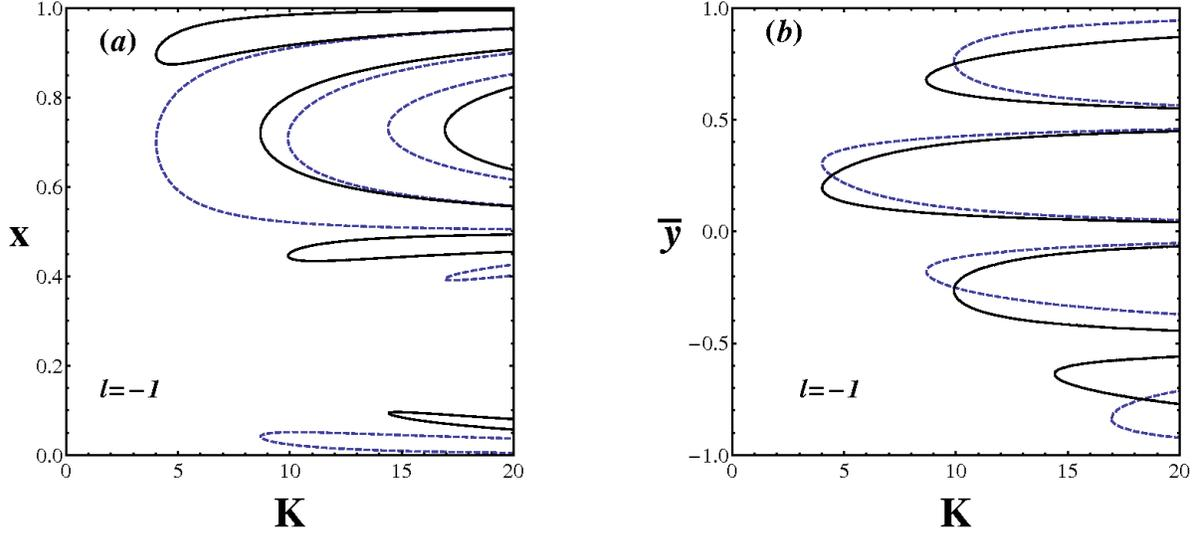
FIG. 13. (a) Characteristics of accelerator mode periodic orbits of period 2, i.e.  $x$  as a function of  $K$  derived from equation (11) for  $l = -1$  (b)  $\bar{y}$  as a function of  $K$  derived from eq. (9) for  $l = -1$ . Black solid curves correspond to equation (11) with the + sign, while (blue in online version) dotted curves correspond to equation (11) with the - sign.
