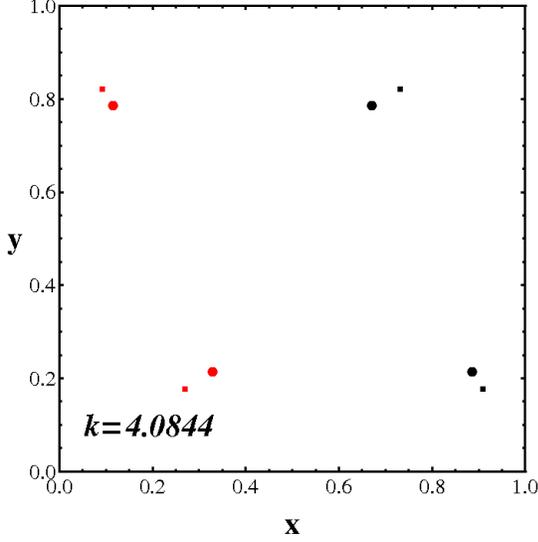
FIG. 15. Four accelerator double periodic orbits for  $K = 4.0844$ . The two black dots represent a stable periodic orbit with modulo 1 both in  $x$  and in  $y$  (black squares correspond to the unstable periodic orbit). The two gray (red in online version) dots represent a second stable orbit with  $x' = 1 - x$  and  $y' = 1 - y$  (gray (red in online version) squares correspond to the unstable periodic orbit).
