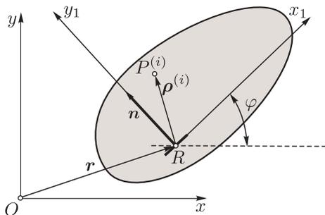
Fig. 2: The Chaplygin sleigh with moving points.
