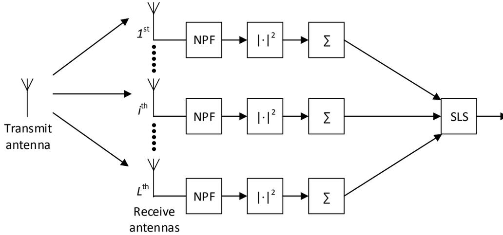
Fig. 2. System model of energy detection for an  $L$ -branch SLS diversity scheme.
