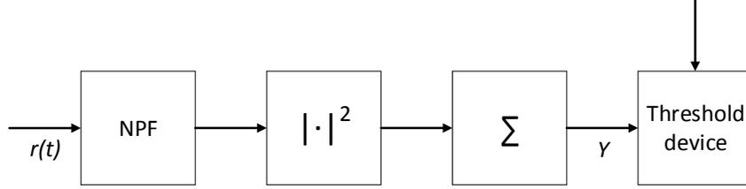
Fig. 1. System model of energy detection.
