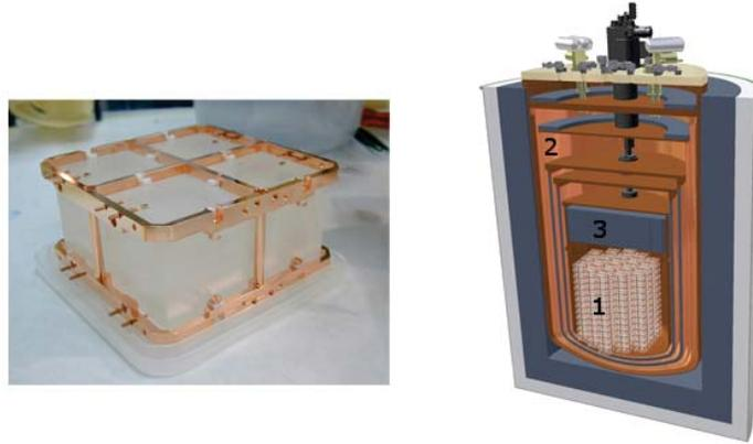
Figure 4.7: On the left side, a floor of a CUORE tower, housing 4  $\text{TeO}_2$  crystals. On the right side, a sketch of the whole CUORE experiment, showing the array of 988  $\text{TeO}_2$  bolometers (1), the dilution cryostat (2), its inner shield made of low-background Roman lead (3).
