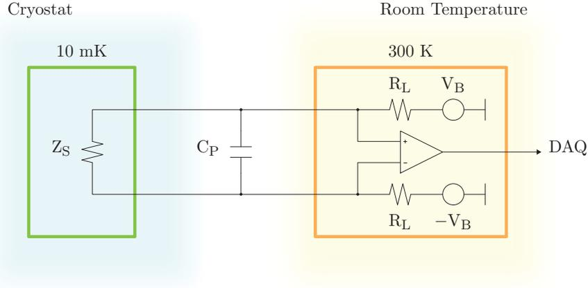
Figure 4.5: Readout of a bolometric sensor at room temperature.
