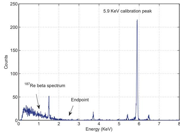
Figure 4.22: A <sup>187</sup>Re beta spectrum recently measured with MARE-1.
