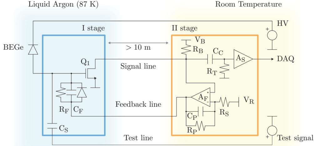
Figure 3.5: Full schematic of the GeFRO circuit.
