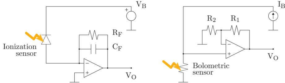
Figure 1.1: Two examples of particle and radiation sensors, including typical biasing and readout circuits. On the left, an ionization sensor readout with a charge amplifier. On the right, a bolometric sensor readout with a voltage amplifier.
