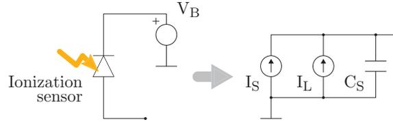
Figure 1.4: Electrical model of a typical ionization sensor.
