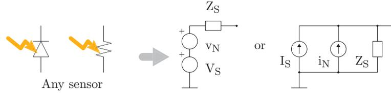
Figure 1.7: General sensor model. For any given sensor, the choice between the two electrical representations on the right is arbitrary.
