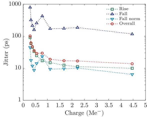
Figure 2.23: Jitter versus input charge in “timing” mode.
