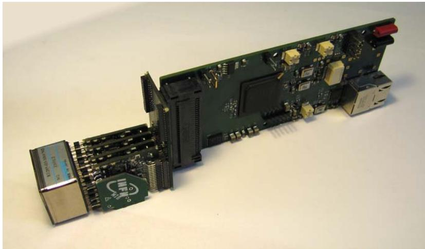
Figure 2.29: Photograph of a R11265 Ma-PMT coupled to the full CLARO-CMOS readout prototype. The high voltage for the Ma-PMT is provided by the smaller PCBs at the sides of the device. On the back, the data acquisition prototype board is shown, developed by S. Wotton of the University of Cambridge.
