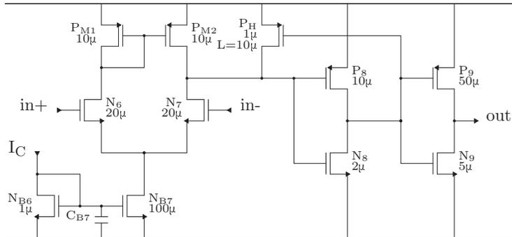
Figure 2.14: Full schematic of the comparator. The width of the MOS transistors is shown. The gate length is  $0.35\ \mu\text{m}$  for all the transistors except  $P_H$ . The substrate of all NMOS (PMOS) transistors is tied to ground (to the positive rail).
