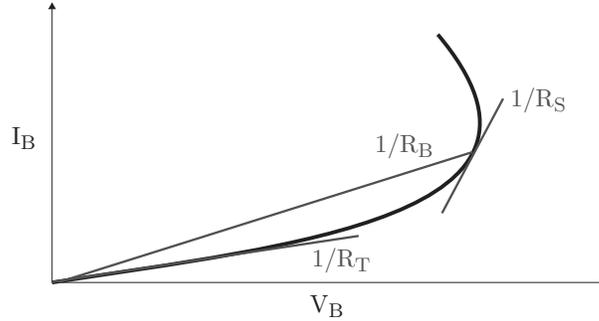
Figure 1.5: Impedance curve of a typical bolometric sensor.
