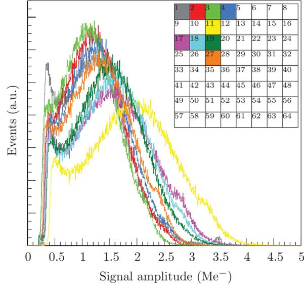
Figure 2.7: Single photon spectra of some pixels of a R11265 Ma-PMT biased at  $-850$  V, with the threshold set at  $300$  Ke $^-$ . The uniformity table provided by Hamamatsu is also shown, where the relative gain between pixels can be found. The colors of the spectra match those of the highlighted pixels in the uniformity table.
