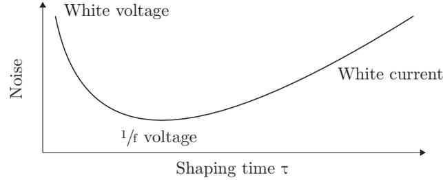
Figure 1.15: Summary of the weight of the noise sources on the signal to noise ratio after a CR – RC<sup>n</sup> filter with time constant  $\tau$  is applied (on top). Qualitative trend of the noise sources versus shaping time (on bottom).
