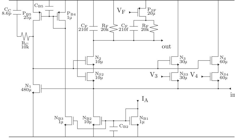
Figure 2.12: Full schematic of the charge amplifier. The width of the MOS transistors is shown. The gate length is  $0.35\ \mu\text{m}$  for all the transistors in the charge amplifier. The substrate of all NMOS (PMOS) transistors is tied to ground (to the positive rail).
