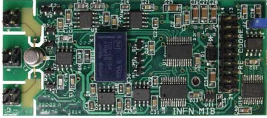
Figure 4.13: Photograph of the front-end amplifier of the CUORE experiment. The PCB is  $80 \times 34 \text{ mm}^2$ . The input JFETs are on the left side, followed by the operational amplifiers, a relay and the DACs. The on-board microcontroller is on the far right.
