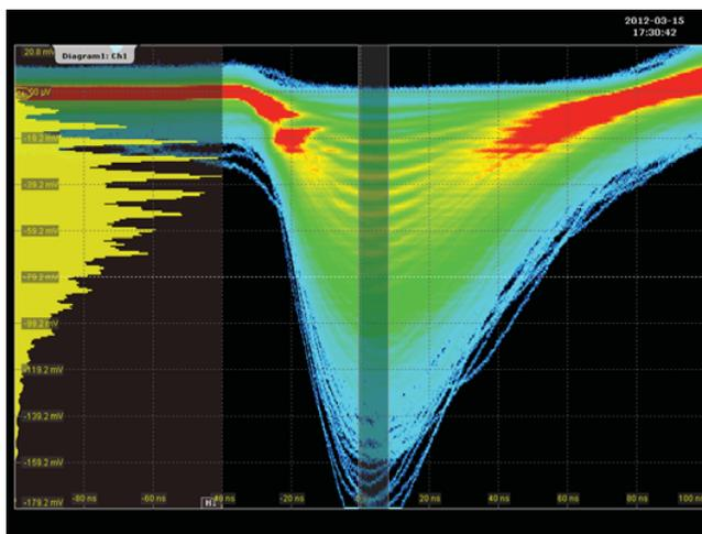
Figure 2.27: Signals at the analog output of a CLARO-CMOS channel with a  $1 \times 1 \text{ mm}^2$  SiPM connected to the input of the ASIC with a coaxial cable 120 cm long. The amplitude histogram is shown on the left side of the oscilloscope screen.
