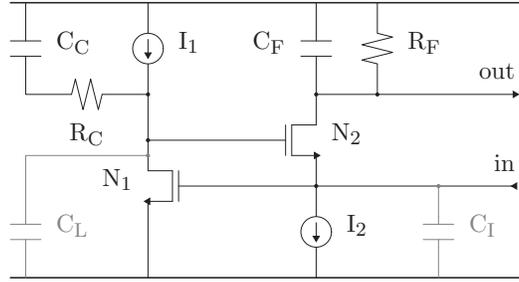
Figure 2.10: Simplified schematic of the charge amplifier.
