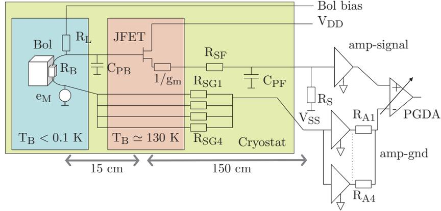
Figure 4.18: Readout scheme of the MARE-1 experiment in Milano.
