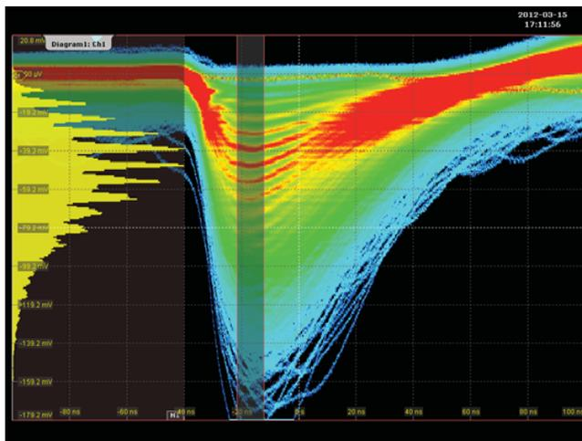
Figure 2.26: Signals at the analog output of a CLARO-CMOS channel with a  $1 \times 1 \text{ mm}^2$  SiPM directly connected to the input of the ASIC. The amplitude histogram is shown on the left side of the oscilloscope screen.
