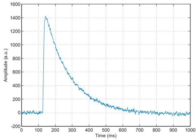
Figure 4.21: A 6 KeV signal from a calibration source.
