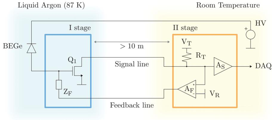
Figure 3.4: Block schematic of the GeFRO circuit.
