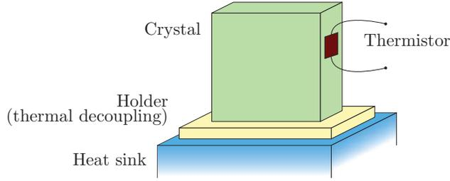
Figure 4.1: Typical setup of a bolometric sensor.
