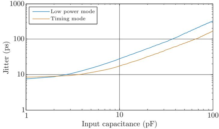
Figure 2.15: Calculated jitter versus input capacitance in “low power” and “timing” modes for  $1 \text{ Me}^-$  signals when the threshold set at  $100 \text{ ke}^-$ .
