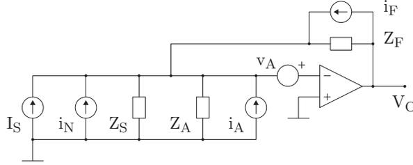
Figure 1.10: General scheme for a sensor readout with a current amplifier, including all the noise sources.
