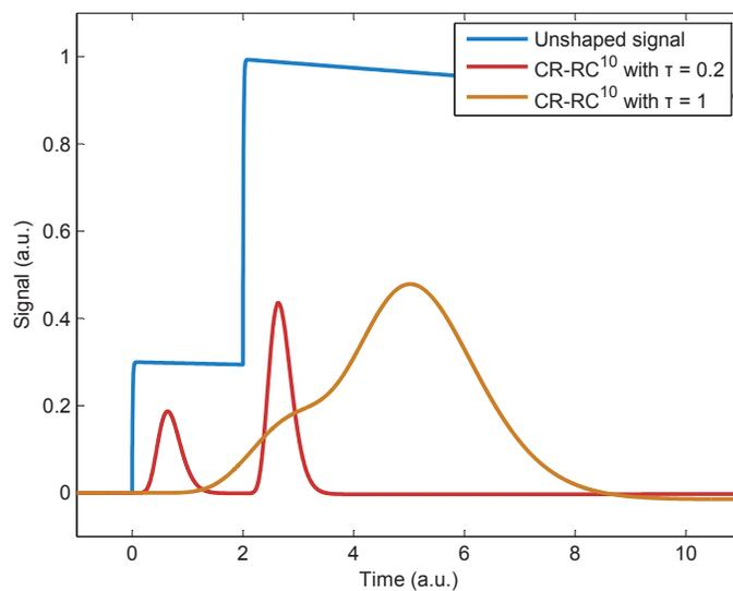
Figure 1.17: Comparison between the unshaped signals with pile-up, the signals shaped with a CR – RC<sup>10</sup> filter with  $\tau = 0.2$  and with a CR – RC<sup>10</sup> filter with  $\tau = 1$ .
