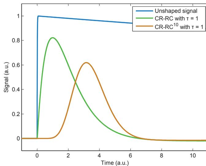
Figure 1.16: Comparison between the unshaped signal, the signal filtered with a CR – RC filter and with a CR – RC<sup>10</sup>, approximating a Gaussian shaping.
