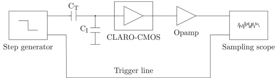
Figure 2.17: Setup used for the CLARO-CMOS performance tests.
