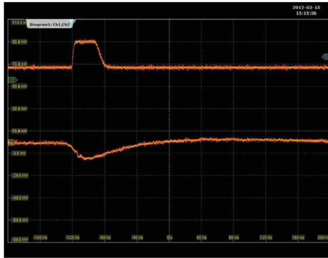
Figure 2.25: Signals at the analog output of a CLARO-CMOS channel with a  $1 \times 1 \text{ mm}^2$  SiPM directly connected to the input of the ASIC. The upper signal is taken at the binary output, the lower signal is taken at the analog output. This is a two photoelectron signal taken just above threshold.
