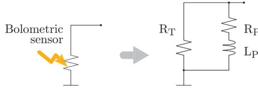
Figure 1.6: Electrical model of a typical bolometric sensor.
