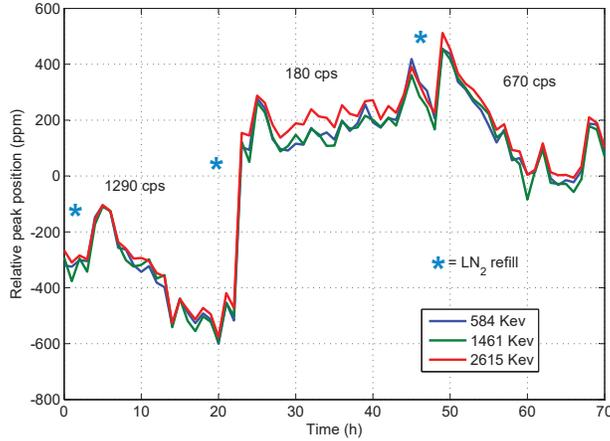
Figure 3.9: Relative peak position versus time over 70 hours of measurement, showing a typical gain drift below 100 ppm/h. The event rate was also changed during the measurement, showing a minimal variation in the position of the peaks.
