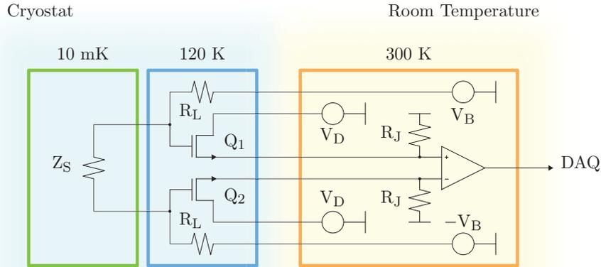
Figure 4.6: Readout of a bolometric sensor at cryogenic temperature.
