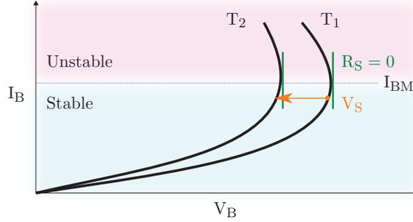
Figure 4.3: The working point of a negative bolometer. When energy is deposited in the bolometer by a particle event, its temperature changes from  $T_1$  to  $T_2$ . The maximum output signal occurs at a bias current  $I_{BM}$ , which also separates the regions of stable and unstable working points.
