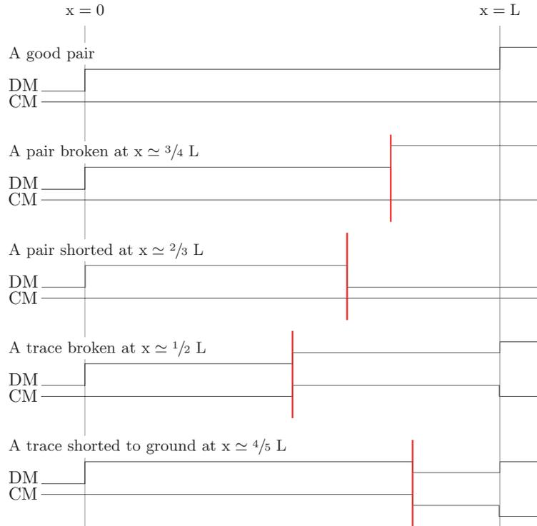
Figure 4.10: Schematic representation of the results of a TDR measurement for a differential pair of traces of length  $L$ , showing the differential mode (DM) and the common mode (CM) reflected waveforms for the case of a good pair (top) and of typical defects.
