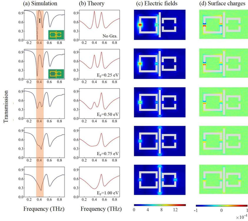
Figure 3: (a) Simulated transmission spectra and corresponding (b) theoretical fitting results, (c) electric field distributions and (d) surface charge distributions at various Fermi levels of monolayer graphene placed under the DSRR1 in the proposed dual-spectral EIT metamaterial.
