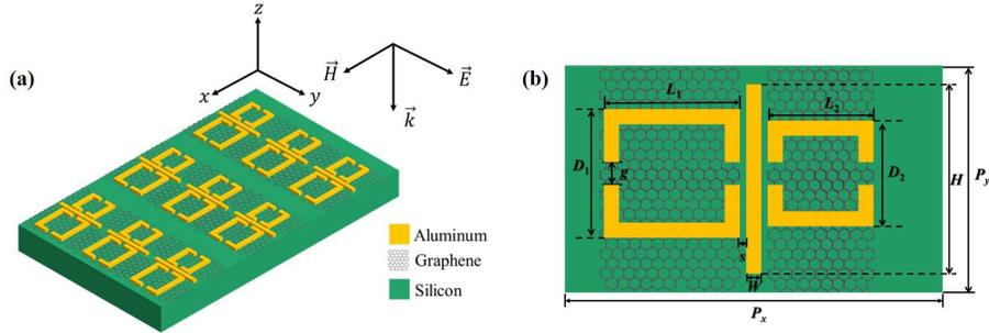
Figure 1: (a) The structural schematic of the proposed hybrid metal-graphene metamaterial and the incident light polarization configuration; (b) the unit cell of the proposed metamaterial,  $P_x = 200 \mu\text{m}$ ,  $P_y = 120 \mu\text{m}$ ,  $H = 100 \mu\text{m}$ ,  $W = 8 \mu\text{m}$ ,  $L_1 = 72 \mu\text{m}$ ,  $L_2 = 56 \mu\text{m}$ ,  $D_1 = 68 \mu\text{m}$ ,  $D_2 = 56 \mu\text{m}$ ,  $g = 12 \mu\text{m}$ ,  $s = 4 \mu\text{m}$ .
