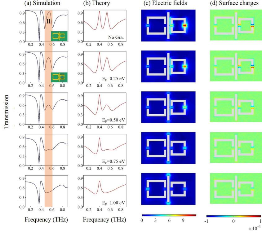
Figure 4: (a) Simulated transmission spectra and corresponding (b) theoretical fitting results, (c) electric field distributions and (d) surface charge distributions at various Fermi levels of monolayer graphene placed under the DSRR2 in the proposed dual-spectral EIT metamaterial.
