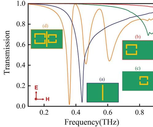
Figure 2: Transmission spectra of the isolated CWR array (blue curve), the isolated DSRR1 array (red curve), the isolated DSRR2 array (green curve) and the combined array (orange curve) under y-polarized electric field.
