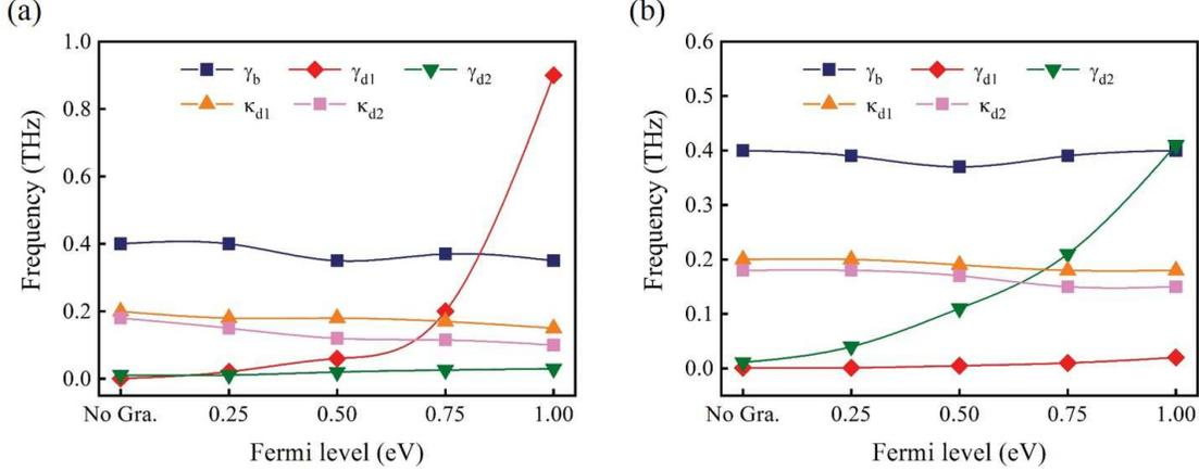
Figure 5: The variations of the fitting parameters including  $\gamma_b$ ,  $\gamma_{d1}$ ,  $\gamma_{d2}$ ,  $\kappa_{d1}$  and  $\kappa_{d2}$  as the function of the Fermi level of graphene placed (a) under the DSRR1 for the modulation of the transmission peak I; (b) under the DSRR2 for the modulation of the transmission peak II in the proposed dual-spectral EIT metamaterial.
