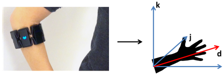
Figure 1: The Myo sensor bracelet used to measure the direction of the arm. The direction of the arm is represented by a three-dimensional unit vector \mathbf{d} .
