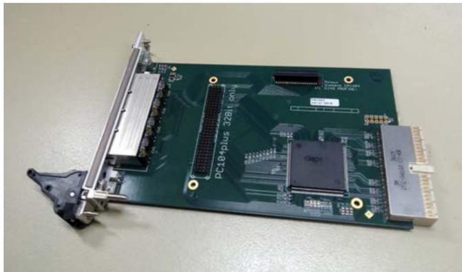
Fig. 6 Photo of the new CompactPCI carrier for PC104+
