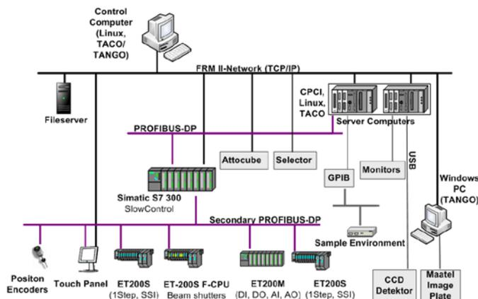
Fig. 1 Physical architecture of the BIODIFF control and DAQ system
