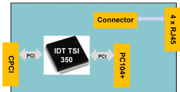
Fig. 5 Simplified block diagram of the new CompactPCI carrier for PC104+
