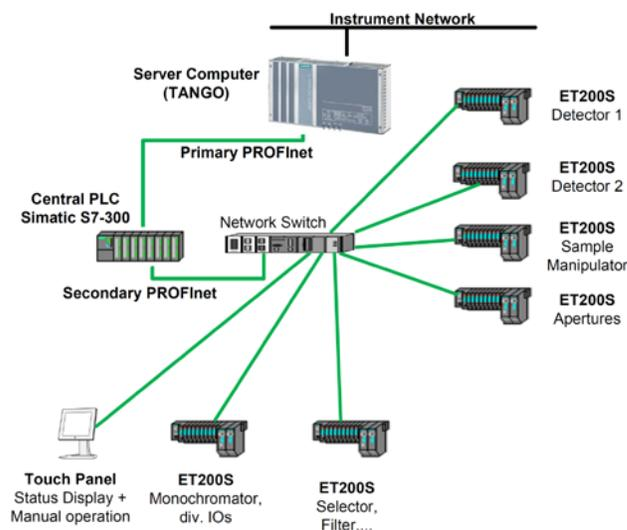
Fig. 4 Physical architecture of the ANTARES motion subsystem
