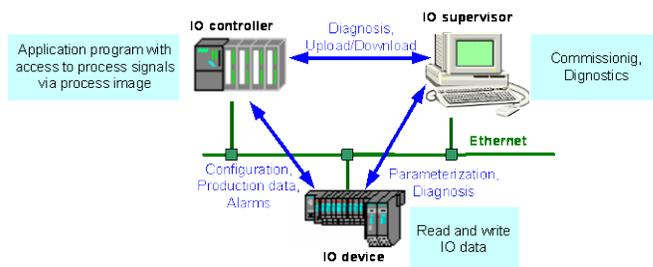
Fig. 2. PROFINET IO communication model
