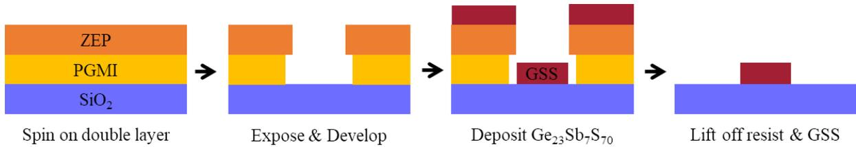
*Fig. 3. Schematic of fabrication process for spiral waveguides. A double layer made of PGMI and ZEP-520A is spun on the oxide wafer. After exposure to e-beam and developing the pattern, we deposit GSS (GeSbS chalcogenide material) and complete the fabrication by lifting off the resist and GSS.*
