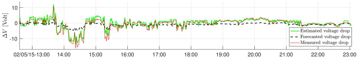
Fig. 10. Comparison of forecasted and estimated voltage with real voltage measurement at the Neighborhood Battery bus.
