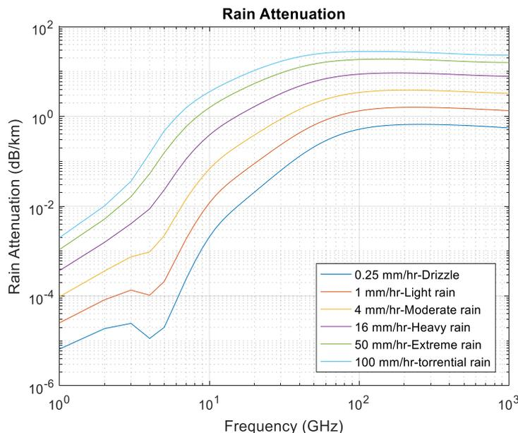
Fig.4. Rain attenuation in dB/Km across the frequency band at different rainfall rates
