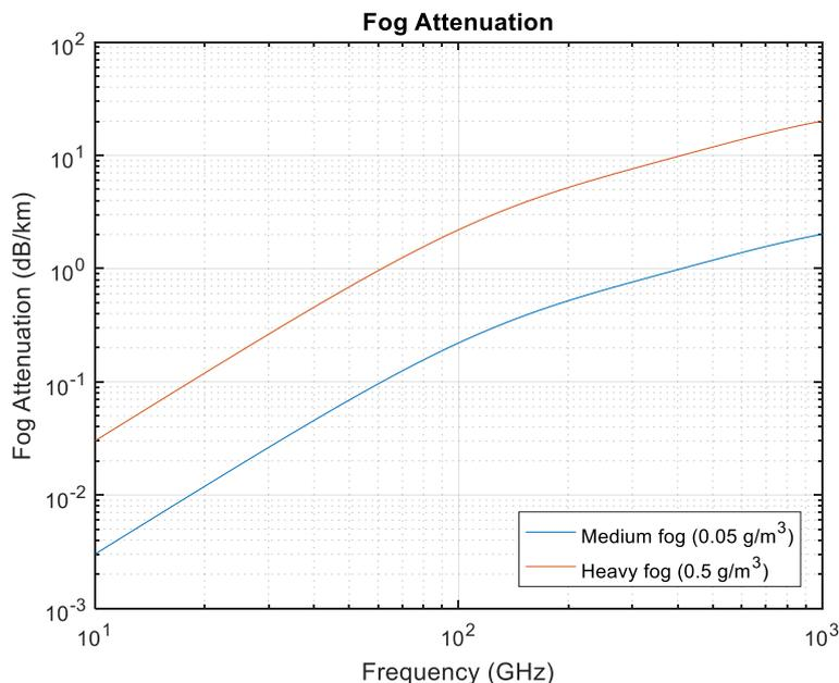
Fig.5. Fog attenuation in dB/Km across the frequency band at different liquid water densities.
