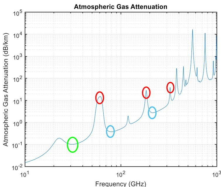
Fig.6. Atmospheric gas attenuation at different frequency bands.
