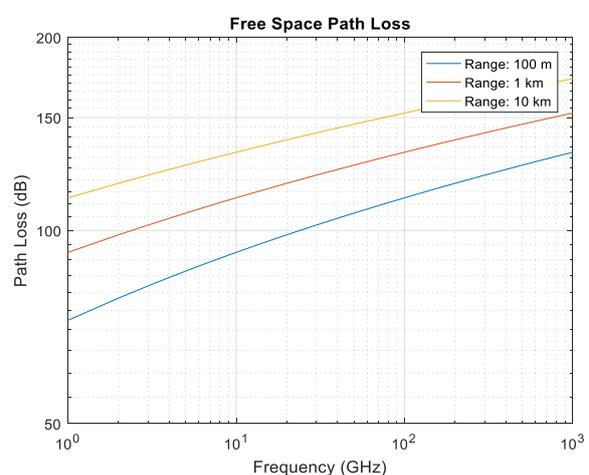
Fig.3. Free space pathloss at T-R distance of 100m, 1Km and 10Km as function of frequency
