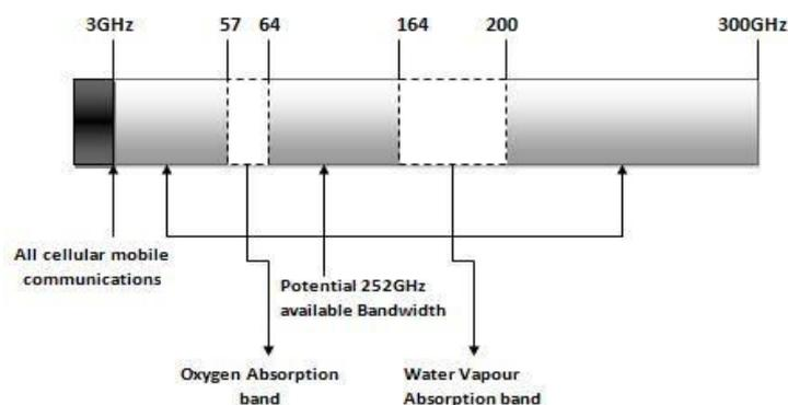
Fig.1. 3GHz-300GHz mm-Wave spectrum
