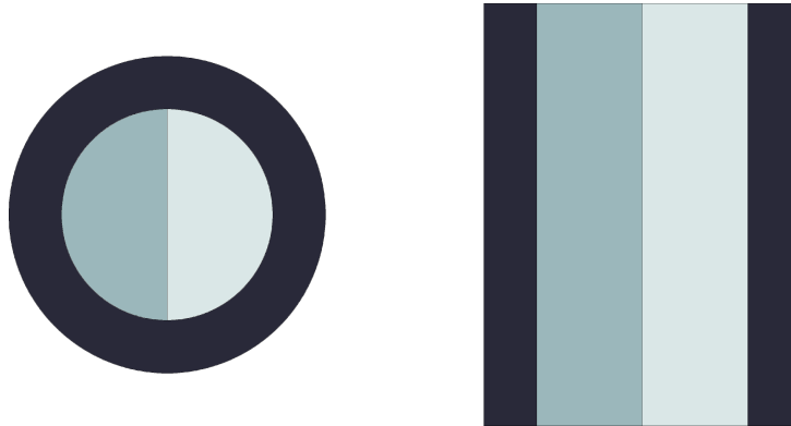
Figure 1: The cylindrical phantom employed to assess the performance of the develop Convex Algorithm Statistical Image Reconstruction (CA-SIR) framework. Inner regions are composed of Titanium (Ti) (left) and Aluminium (Al) (right) half cylinders of 10 mm in radius and 40 mm height, with a Stainless Steel (S.S.) outer shell 5 mm thick and 40 mm in height. The colour scale used represents the three materials linear attenuation coefficient at the maximum intensity of DINGOs Maxwell-Boltzmann distributed thermal spectrum ( 1.5 \text{ \AA} ): S.S. 1.131 \text{ cm}^{-1} , Al 0.101 \text{ cm}^{-1} , and Ti 0.450 \text{ cm}^{-1} [22, 23].
