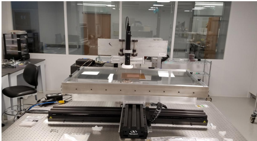
Figure 5: CCD camera and 2D stage capable of scanning areas up to 100 \times 80 \text{ cm}^2 . This image shows a 10 \times 10 \text{ cm}^2 GEM foil that is being scanned.
