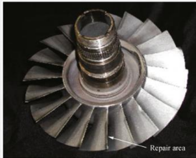
Figure 12: Damaged area repaired with LENS process
