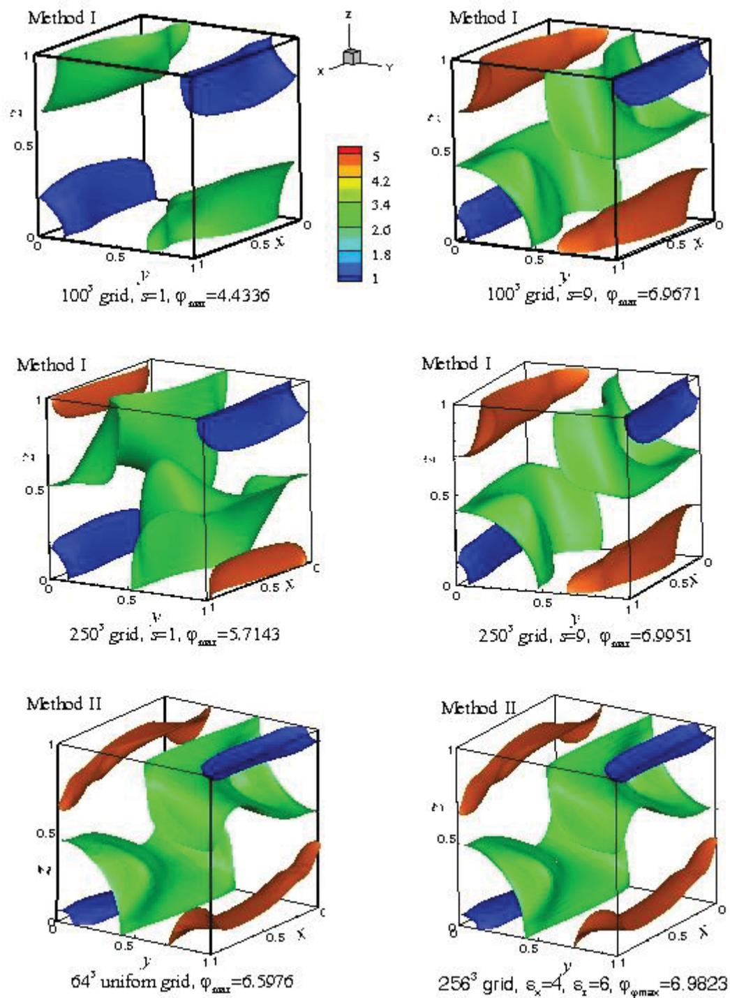
**Figure 7.** Equipotential surfaces for  $Pr=0.054$ ,  $Ra=10^6$ ,  $Ha_z=100$  calculated on different grids with different stretching by the Methods I and II. The levels  $\varphi = 2.0, 4.0$  and  $6.0$  are shown.
