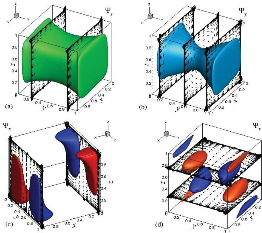
**Figure 12.** Visualization of the velocity field for  $Ha_x = 100$  by vector potentials of divergence free velocity projections. Maximum and minimum values of the velocity potentials are: (a,b)  $-0.0465, 0.000300$ ; (c)  $\pm 0.00825$ ; (d)  $\pm 0.00370$ . Levels plotted are: (a)  $-0.021$ ; (b)  $-0.029$ ; (c)  $\pm 0.003$ ; (d)  $\pm 0.0022$ .
