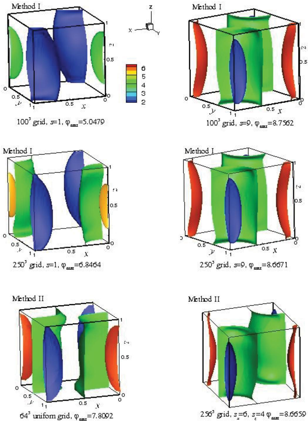
**Figure 6.** Equipotential surfaces for  $Pr=0.054$ ,  $Ra=10^6$ ,  $Ha_x=100$  calculated on different grids with different stretching by the Methods I and II. The levels  $\varphi = 2.0, 4.0$  and  $6.0$  are shown. In this figure and in figures 7 and 8, the free additive constant in the definition of the potential is fixed by setting the minimum value of  $\varphi$  to zero.
