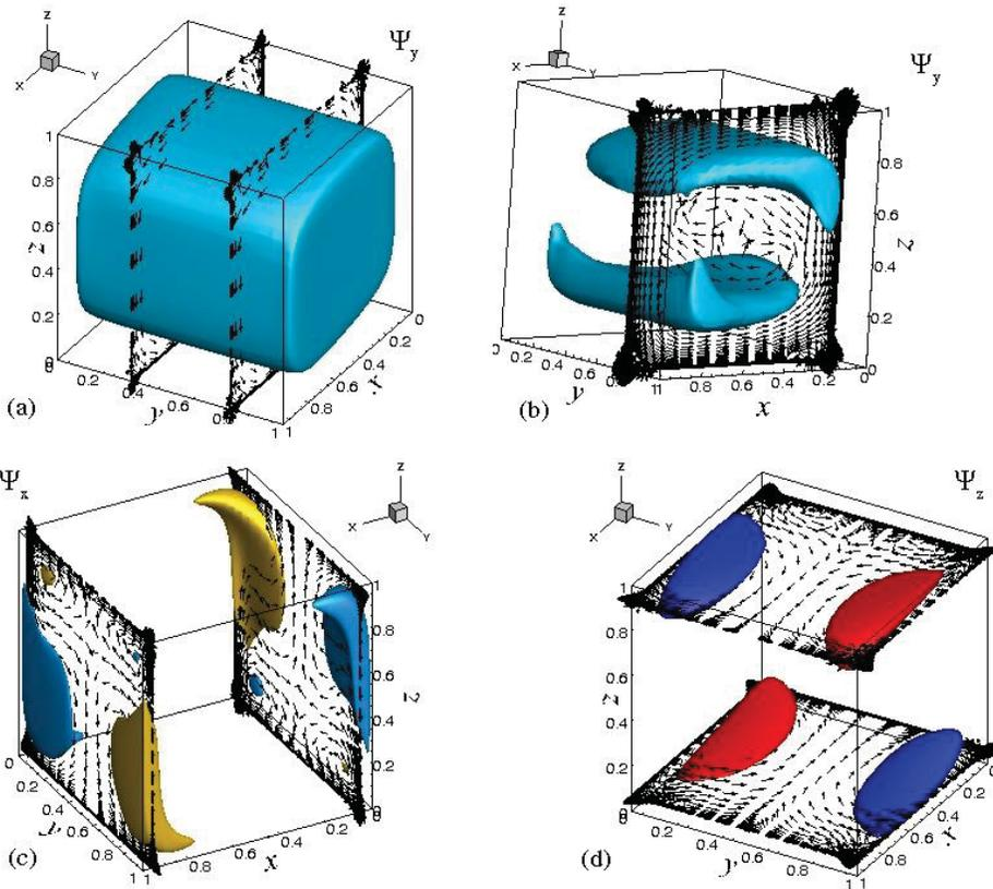
**Figure 14.** Visualization of the velocity field for  $Ha_y = 100$  by vector potentials of divergence free velocity projections. Maximum and minimum values of the velocity potentials are: (a,b) -0.0510, 0.00571; (c)  $\pm 0.00642$ ; (d)  $\pm 0.0101$ . Levels plotted are: (a) -0.04; (b) -0.048; (c)  $\pm 0.002$ ; (d)  $\pm 0.006$ .
