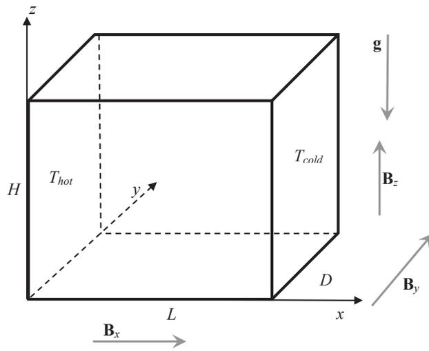
**Figure 1.** Sketch of the considered flow configuration. Laterally heated three-dimensional cubic box under the effect of external magnetic field of three possible directions.
