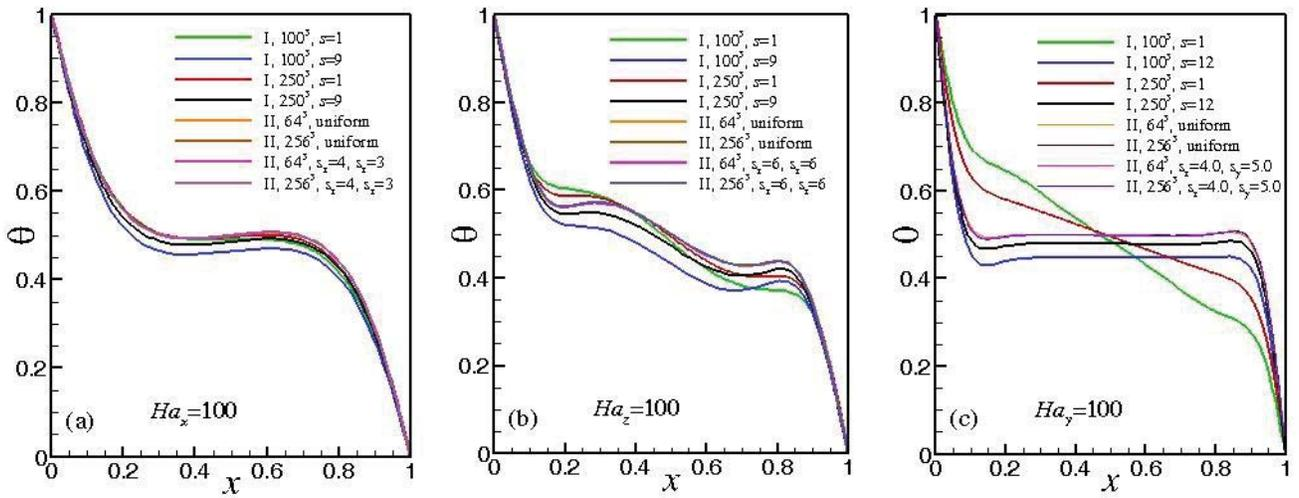
**Figure 9.** Temperature profiles along the line  $y = z = 0.5$  in flows with three different orientations of the magnetic field, on different grids with different stretching computed by the Methods I and II.
