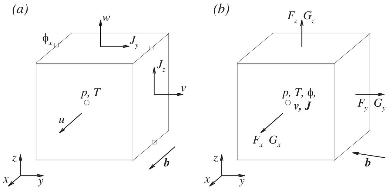
**Figure 2.** Illustrations of the grid arrangement systems used in the study. (a), The fully staggered grid applied in the Method I in the case of the magnetic field  $\mathbf{b} = \mathbf{e}_x$ . (b), The collocated grid applied in the Method II for an arbitrary magnetic field  $\mathbf{b}$ .
