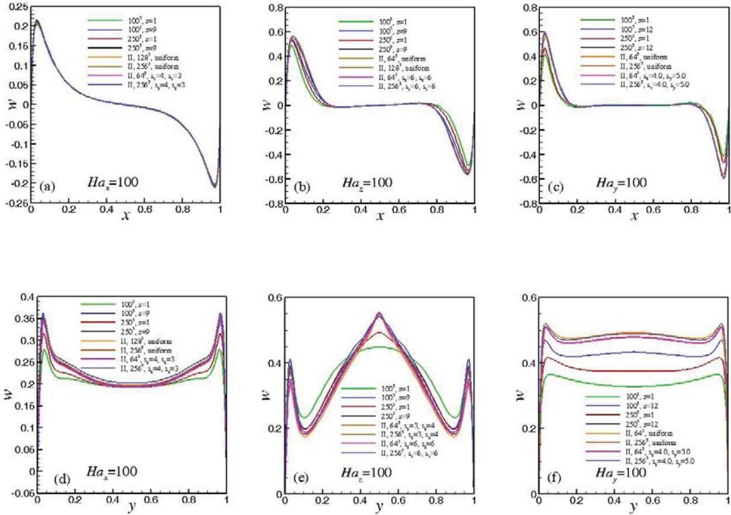
**Figure 11.** Profiles of the  $z$ -component of velocity  $w$  in flows with three different orientations of the magnetic field computed on different grids with different stretching by the Methods I and II. The profiles are drawn along the lines (a) – (c)  $y = z = 0.5$ , (d) – (f)  $x = 0.05, z = 0.5$ .
