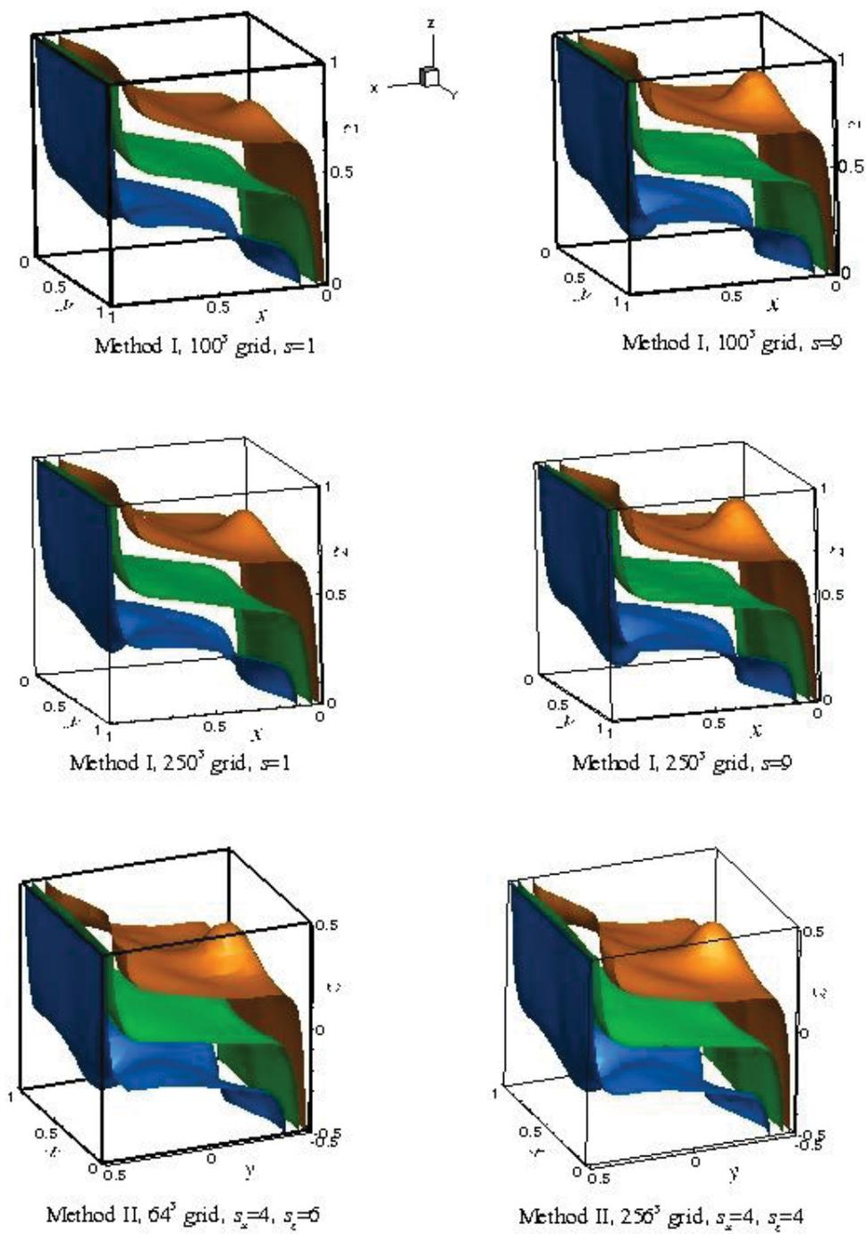
**Figure 4.** Isotherms  $\theta = 0.1, 0.5,$  and  $0.9$  for  $Pr=0.054, Ra=10^6, Ha_z=100$  calculated on different grids with different stretching by the Methods I and II.
