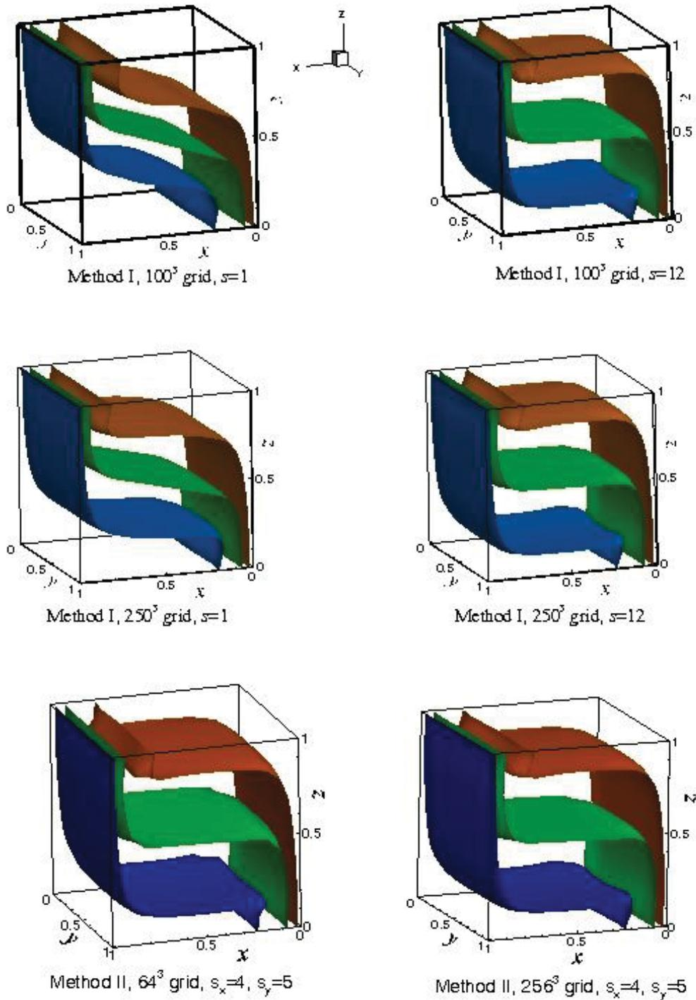
**Figure 5.** Isotherms  $\theta = 0.1, 0.5$ , and  $0.9$  for  $Pr=0.054$ ,  $Ra=10^6$ ,  $Ha_y=100$  calculated on different grids with different stretching by the Methods I and II.
