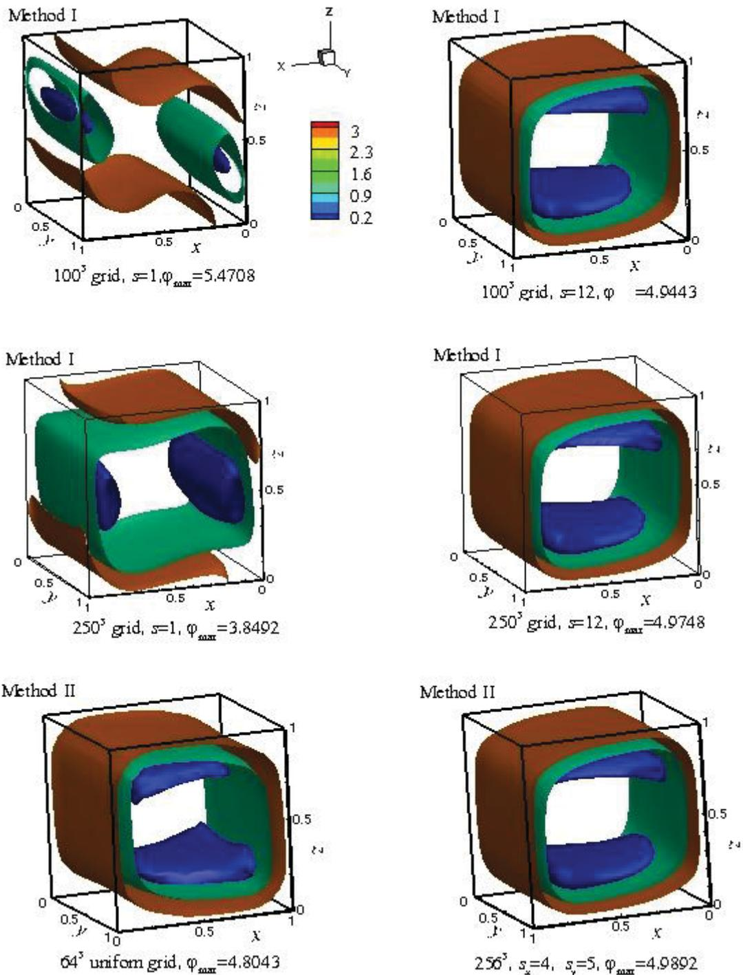
**Figure 8.** Equipotential surfaces for  $Pr=0.054$ ,  $Ra=10^6$ ,  $Ha_y=100$  calculated on different grids with different stretching by the Methods I and II. The levels  $\varphi = 2.0, 4.0$  and  $6.0$  are shown.
