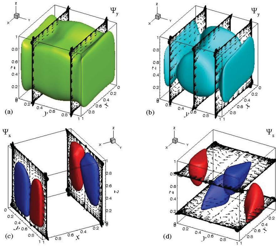
**Figure 13.** Visualization of the velocity field for  $Ha_z = 100$  by vector potentials of divergence free velocity projections. Maximum and minimum values of the velocity potentials are: (a,b)  $-0.0584, 0.00504$ ; (c)  $\pm 0.0251$ ; (d)  $\pm 0.0105$ . Levels plotted are: (a)  $-0.0122$ ; (b)  $-0.0266$ ; (c)  $\pm 0.025$ ; (d)  $\pm 0.007$ .
