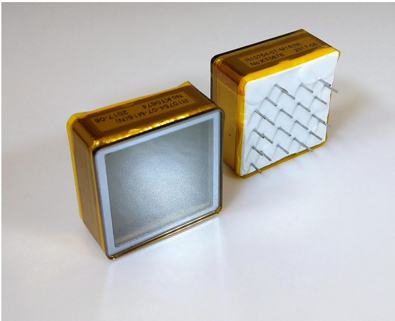
Figure 5: 16-pixel Hamamatsu R10754-07-M16(N) microchannel plate photomultiplier tube. The dimensions are 27.6 x 27.6 x 13.1 mm 3 without pin wires and 27.6 x 27.6 x 16.7 mm 3 with pin wires.
