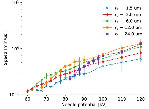
**Figure 19.** Streamer propagation speed for a series of different streamer head tip curvatures  $r_s$ . The dotted lines are interpolated to the average, and the bars covers the minimum and maximum values.
