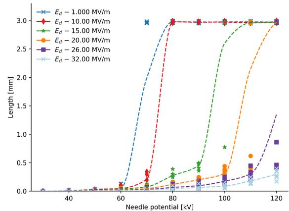
**Figure 14.** Streamer propagation length as a function of needle potential and electron detachment threshold  $E_d$ . Each marker is a simulation and the dotted lines are interpolated to the average.
