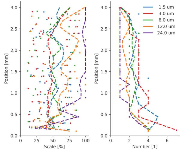
**Figure 20.** Actual streamer head scale  $k_i$  (left) and total number of streamer heads (right) at 100 kV for a series of streamer head tip curvatures  $r_s$ . Data are taken every 5 % of the gap. The dashed lines are moving averages calculated by loess-regression [72].
