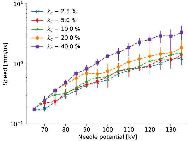
**Figure 21.** The effect of streamer head scale threshold  $k_c$  on the streamer propagation speed, calculated for the mid 50 % of the gap. The dotted lines are interpolated to the average, and the bars covers the minimum and maximum values.
