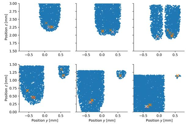
**Figure 28.** Detailed illustration of streamer branching. The electron avalanches are shown as blue dots, and the streamer head as crosses. The top three plots show streamer bifurcation in the start of the gap, while the bottom three plots show one propagating branch and another stopped branch at the end of the gap.
