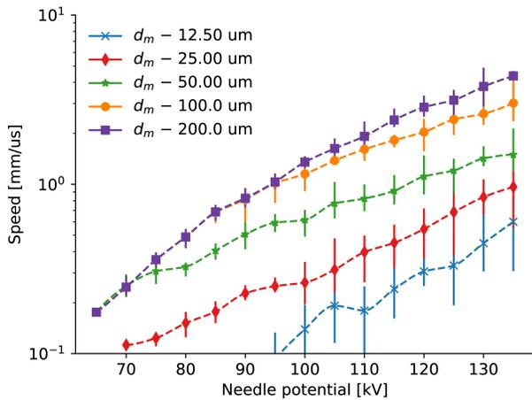
**Figure 22.** The effect of streamer merge distance  $d_m$  on the streamer propagation speed, calculated for the mid 50 % of the gap. The dotted lines are interpolated to the average, and the bars covers the minimum and maximum values.
