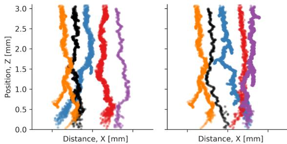
**Figure 23.** Streamer head positions for simulations at 120 kV. Variation of  $k_c$  (left): 10 % (yellow), 20 % (black), 2.5 % (blue), 5.0 % (red), and 40 % (purple). Variation of  $d_m$  (right): 50.0  $\mu\text{m}$  (yellow), 200  $\mu\text{m}$  (black), 25.0  $\mu\text{m}$  (blue), 100  $\mu\text{m}$  (red), and 12.5  $\mu\text{m}$  (purple).
