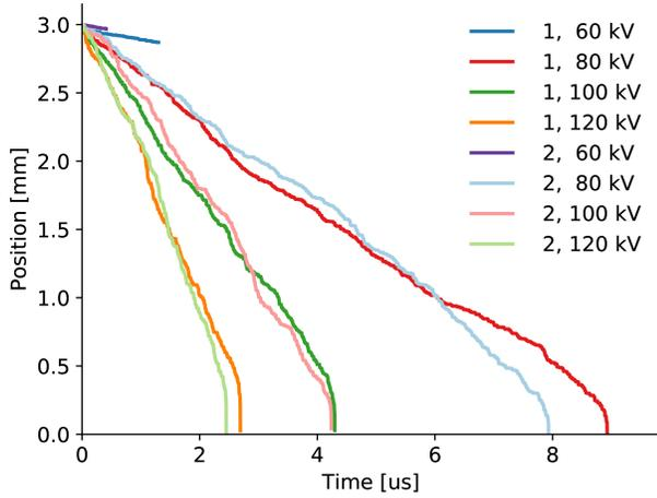
**Figure 7.** Streak plots, time spent versus leading head position, for two simulations (different initial random numbers) at each voltage. The streamers start at the position of the needle,  $z = d_g = 3.0$  mm.
