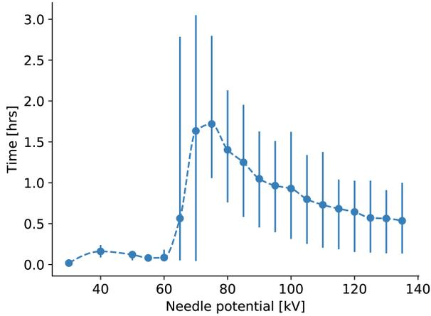
**Figure 30.** Total computational time for the simulations shown in figure 21. Streamers that terminate in the beginning of the gap require little time, while streamers that slowly bridge the gap requires the most computational time.
