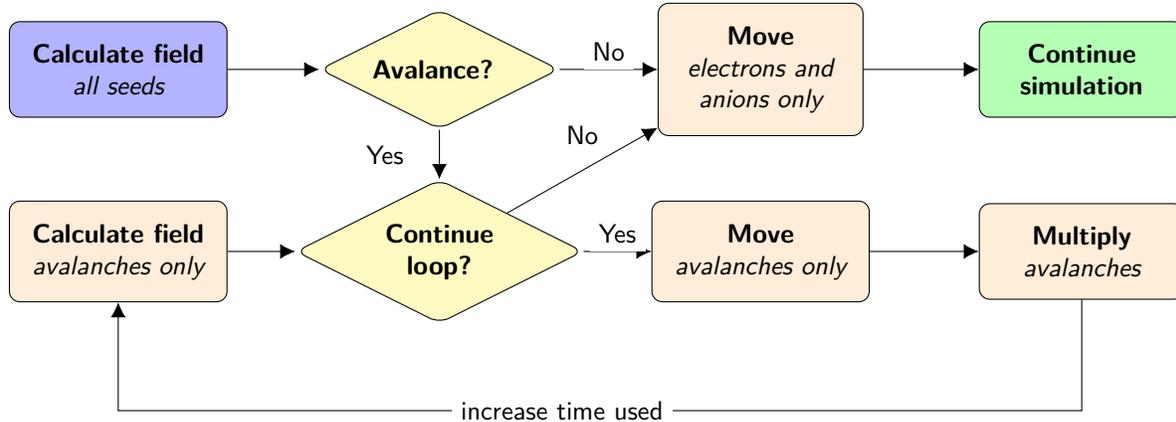
**Figure 6.** Algorithm for moving and multiplying seeds. This is the block labeled “Seeds” in figure 5. See section 2.8 for details on each step.
