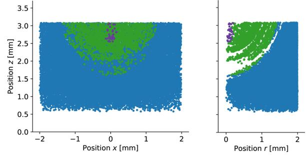
**Figure 13.** Streamer stop after sweep-out of too many electrons at 90 kV and  $E_d = 15 \text{ MV m}^{-1}$ .  $xz$ - and  $rz$ -projection where each seed is represented by a dot; anion (blue), electrons (green), and avalanches (purple).
