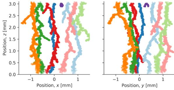
**Figure 26.** Streamer trails for a range of voltages, using the same colors as in figure 25. Each dot represents the position of a streamer head at some point of the propagation.
