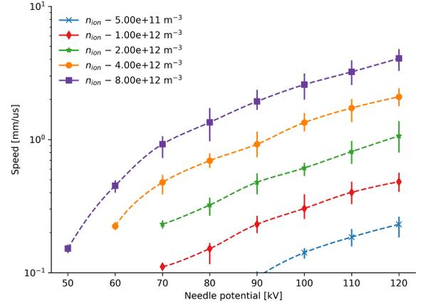
**Figure 12.** The effect of seed concentration  $n_{\text{ion}}$  on the average streamer propagation speed for the middle 50 % of the gap. Streamers terminated in the first 25 % of the gap are excluded. The default concentration is about  $2 \times 10^{12} \text{ m}^{-3}$ . The dashed lines are interpolated to the average, and the bars covers the minimum and maximum values.
