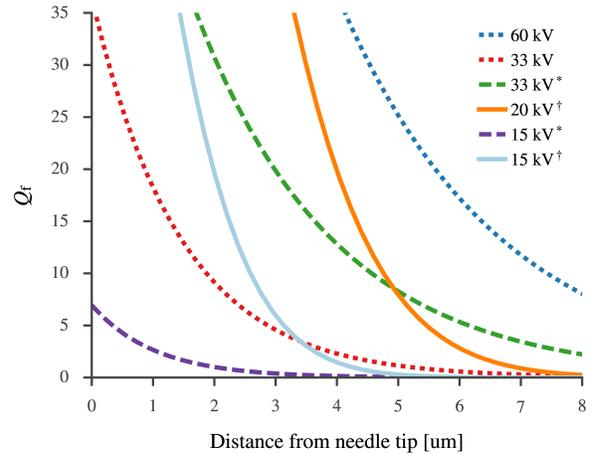
**Figure 29.** Maximum avalanche size at a distance from the needle tip. The unmarked lines use the same values as the baseline simulations from [22], the \* indicates parameter values from [62] as used in section 3.5, and the † indicates formulation and parameter values from [61].
