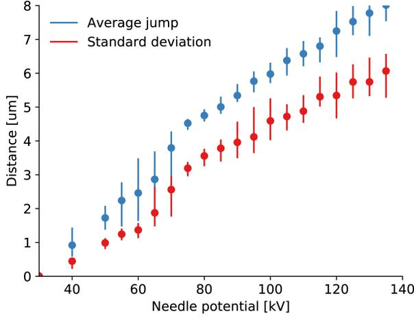
**Figure 11.** The leading streamer head is moved in a sequence of discrete “jumps” in the  $z$ -direction. The average jump length and the standard deviation of the jumps are found for each individual simulation. The dotted lines are interpolated to the average, and the bars covers the minimum and maximum values for ten simulations at the same voltage.
