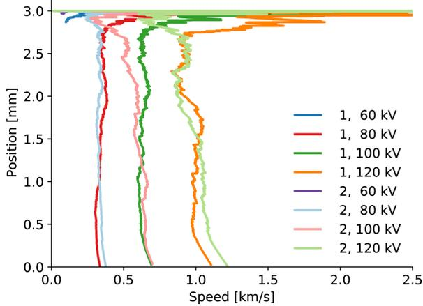
**Figure 8.** Streamer average speed versus leading head position, that is, the average gradient of the “streaks” shown in figure 7.
