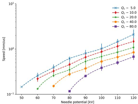
**Figure 16.** The effect of  $Q_c$  on the average streamer propagation speed for the middle 50 % of the gap. The dashed lines are interpolated to the average, and the bars covers the minimum and maximum values.
