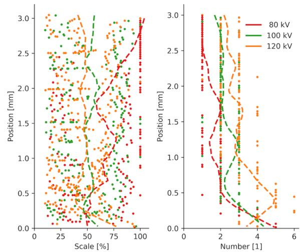
**Figure 10.** Actual streamer head scale  $k_i$  (left) and total number of streamer heads (right). Data are taken every 1% of the gap. The dashed lines are moving averages calculated by loess-regression [72].
