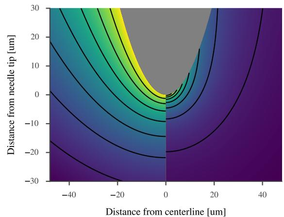
**Figure A2.** Electric potential (left) and electric field strength (right), for a region close to a needle (center, gray) placed 10 mm from a grounded plane. The contour lines give a qualitative impression of how the respective magnitudes change as a function of position. A linear scale is used for both sides, and the magnitudes are linearly dependent on the potential of the needle.
