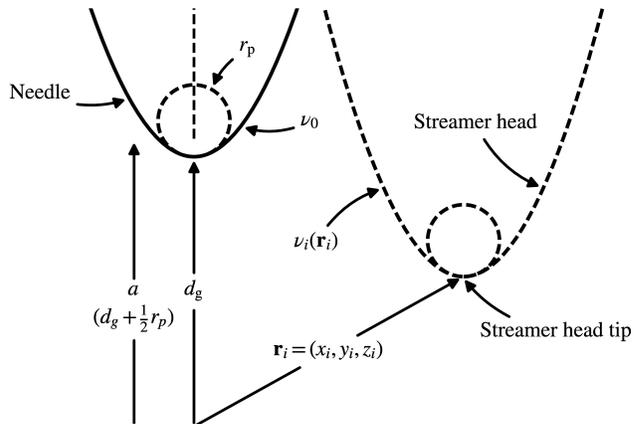
**Figure 1.** The hyperbolic needle and a streamer head, with relevant variables shown. The distance to the plane is usually far greater than illustrated here.
