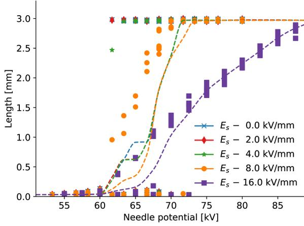
**Figure 17.** Streamer propagation length as a function of needle potential and electric field in streamer channel  $E_s$ . Each marker is a simulation and the dotted lines are interpolated to the average. Note that up to  $8 \text{ kV m}^{-1}$ , the results overlap to a high degree.
