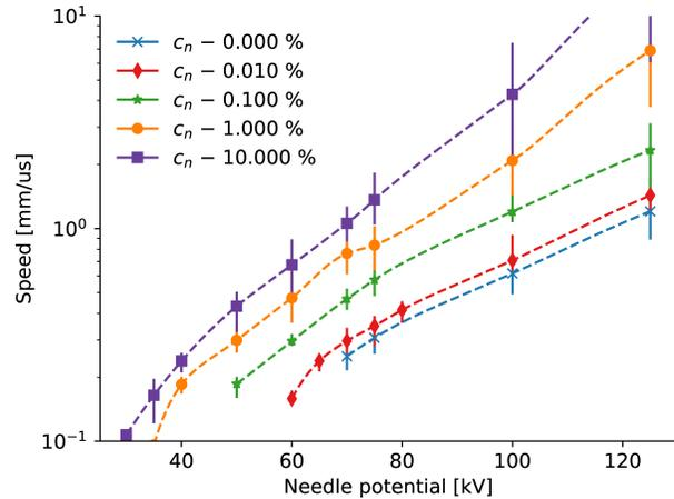
**Figure 24.** Streamer propagation speed for various fractions of added additive  $c_n$ . Average speed for the middle 50 % of the gap. Each marker is a simulation and the dotted lines are interpolated to the average.
