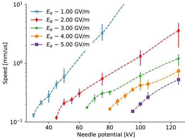
**Figure 15.** The effect of  $E_\alpha$  on the average streamer propagation speed for the middle 50 % of the gap. The dashed lines are interpolated to the average, and the bars covers the minimum and maximum values.
