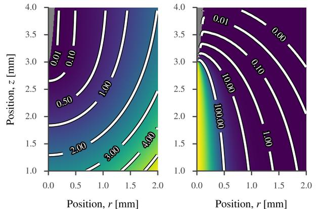
**Figure 4.** Time to collision  $t_i$  (left, in milliseconds) and maximum avalanche size  $Q_i$  (right), for an electron originating at a given position. The needle hyperbola is shown in gray. For a gap distance of 3 mm, a tip radius of 6  $\mu\text{m}$ , and at a potential of 100 kV.
