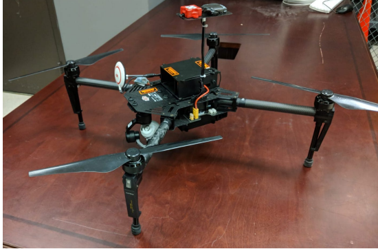
Figure 7: DJI Matrice 100 quadcopter used for data collection
