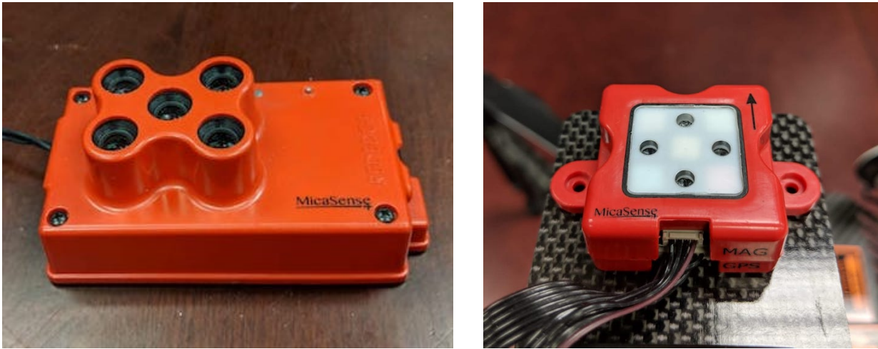
(a) (b) Figure 3: MicaSense RedEdge (a) camera, and (b) downwelling light sensor
