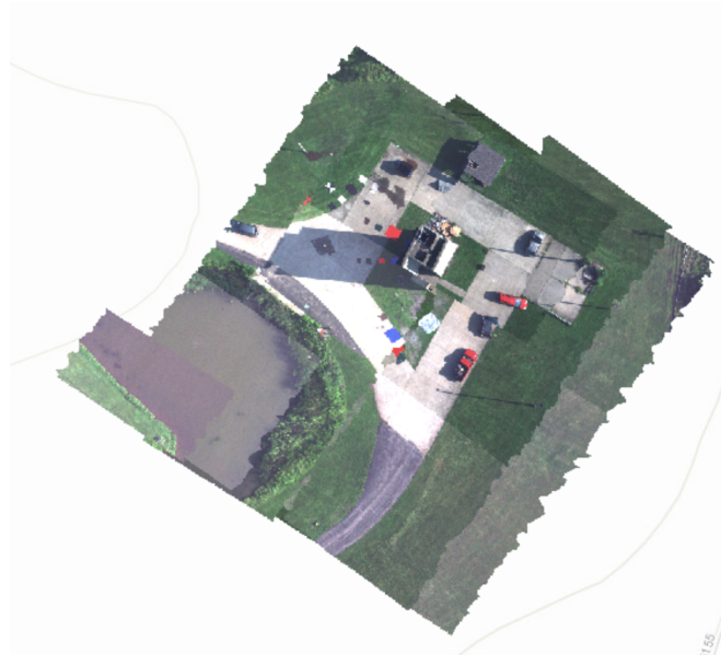
Figure 6: Henrietta Fire District Training Center orthomosaiced image. Calibration panels and test felts are distributed throughout the scene (in direct sunlight and shadow regions).
