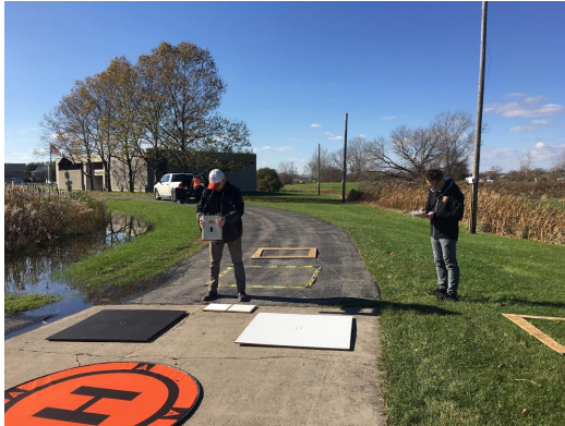
Figure 8: Example spectra collection in the field. Note that collector’s shoulder is towards the sun. Measurements account for non-uniformity in the target by averaging an area of collection.
