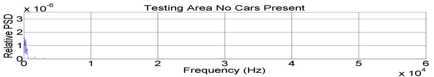
Figure 3. PSD of a the testing area with no cars present
