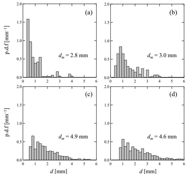
FIG. 10. Fragment-diameter distribution histograms for (a) Case 1 ( $D_{j0} = 7 \text{ mm}$ ), (b) Case 2 ( $D_{j0} = 10 \text{ mm}$ ), (c) Case 3 ( $D_{j0} = 15 \text{ mm}$ ), and (d) Case 4 ( $D_{j0} = 20 \text{ mm}$ ). Here,  $d_m$  denotes the mass-median diameter. Larger inlet diameter  $D_{j0}$  lead to large fragments appearing more frequently.
