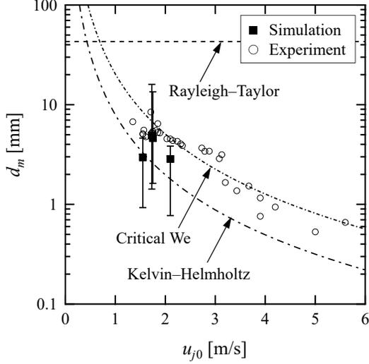
FIG. 11. Comparison of the experimental and simulated fragment sizes. Here, the critical Weber number  $We_{cr}$  in Eq. (52) was assumed to be 18. Both the experimental [23] and simulation results are in accordance with the Kelvin-Helmholtz [Eq. (51)] and critical Weber number [Eq. (52)] theories. However, the Rayleigh-Taylor instability [Eq. (50)] does not correlate with either the numerical or experimental results.
