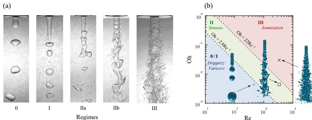
FIG. 1. (a) Snapshots of typical jet breakup regimes in liquid–liquid systems: dripping (0), varicose (I), sinuous *without* entrainment (IIa), sinuous *with* entrainment (IIb), and atomization (III) [13]. (b) Map of jet breakup regimes in immiscible liquid–liquid systems [13, 14]
