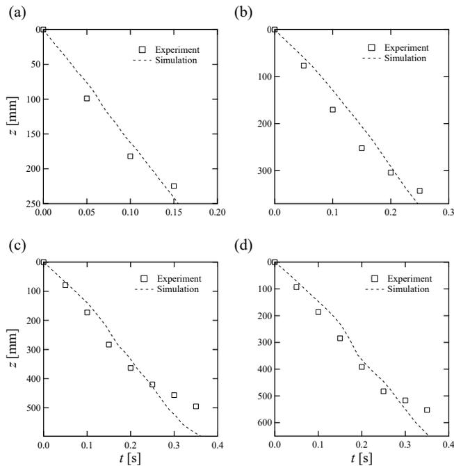
FIG. 9. Evolution of the jet's leading edge over time for (a) Case 1 ( $D_{j0} = 7 \text{ mm}$ ), (b) Case 2 ( $D_{j0} = 10 \text{ mm}$ ), (c) Case 3 ( $D_{j0} = 15 \text{ mm}$ ), and (d) Case 4 ( $D_{j0} = 20 \text{ mm}$ ). In all cases, the experimental observations are ahead of the simulation early on, but the simulation passes the experiment in the latter stages. Overall, the simulations reproduce the experimental trends well.
