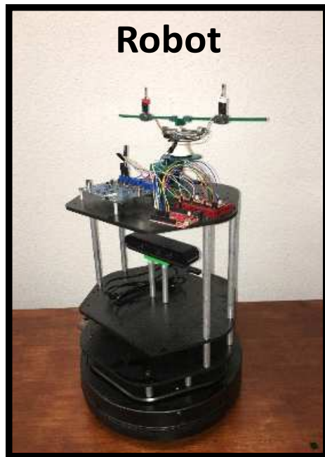
Fig. 6: Kobuki Turtlebot robot with the platform mounted with two microelectromechanical systems (MEMS) microphones.
