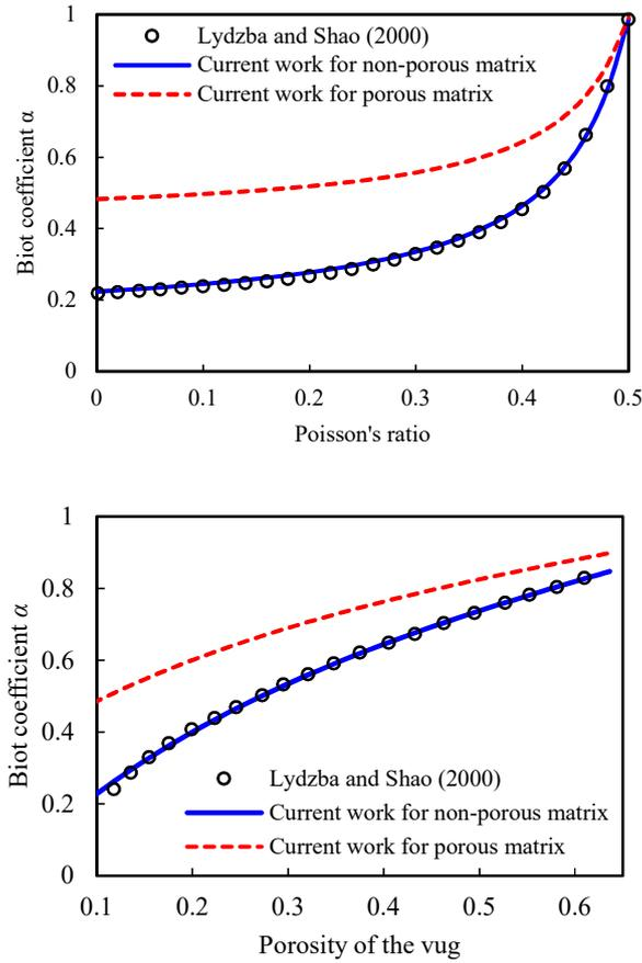
**Figure 5: Biot coefficient  $\alpha_{11}$  versus Poisson's ratio (top) and porosity of the vug (bottom).**
