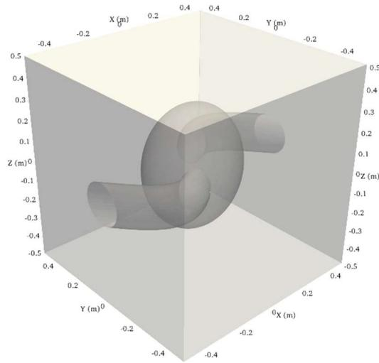
Figure 8: 3D Geometry of a porous medium with a tortuous vug
