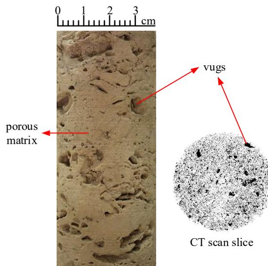
**Figure 1: A typical core of vuggy carbonate reservoirs.**
