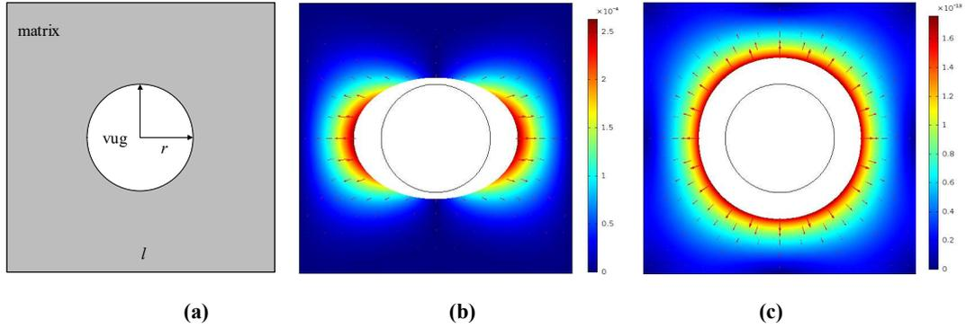
**Figure 4: (a) Schematic of a porous medium with a circular vug, (b) the solution  $\xi^{11}$  of base problem (21) corresponding to the x-direction displacement, (c) the solution  $\zeta$  of base problem (22) corresponding to the total displacement results.**
