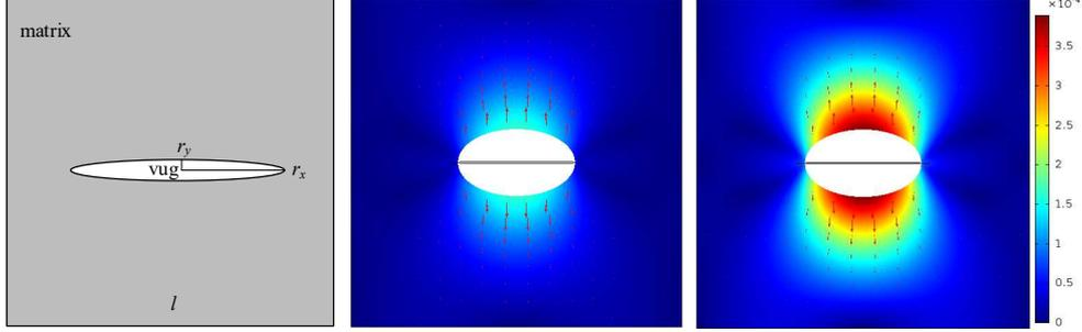
**Figure 6: (a) Schematic of a porous medium with a penny-shaped vug, (b) the solution  $\xi^{11}$  of base problem (21) corresponding to the total displacement, (c) the solution  $\xi^{22}$  of base problem (21) corresponding to the total displacement results.**
