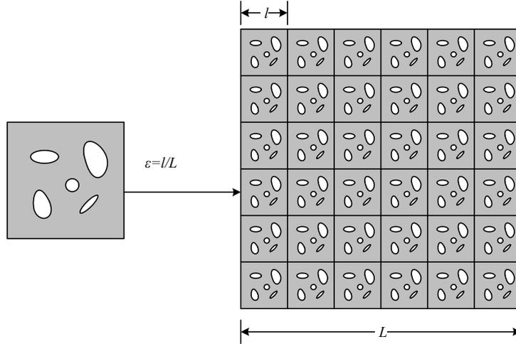
Figure 3: Schematic of a periodic vuggy porous medium
