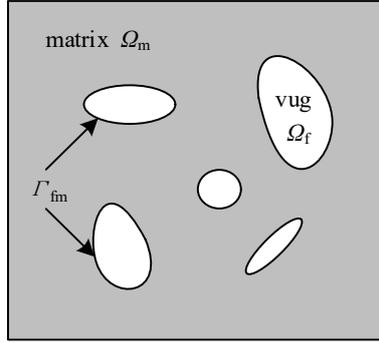
Figure 2: Schematic of a periodic porous medium with micro vugs.
