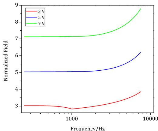
**Figure 5.** Frequency dependence of the magnetic field generated by the driving coil at different applied voltages. The curves have been normalized relative to the data at 1 V.
