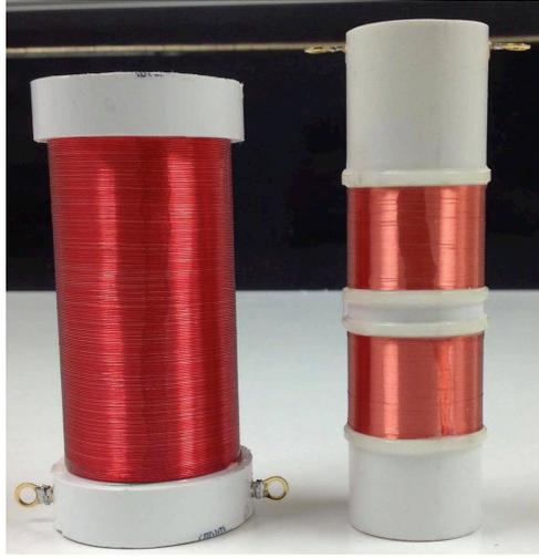
**Figure 3.** Driving coil (left) and pick-up coil (right).
