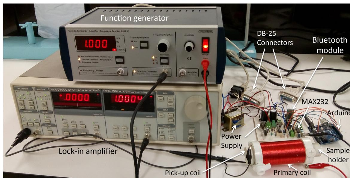
**Figure A2.** Instrumentation assembly.
