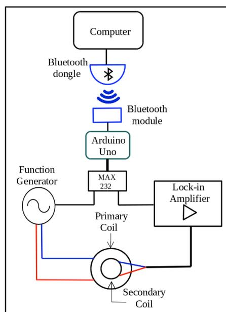
**Figure 1.** Block diagram for the susceptometer.
