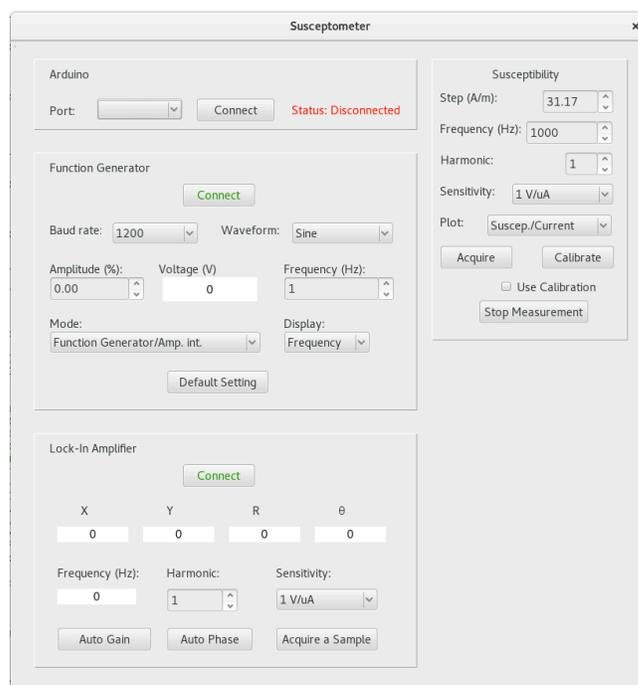
**Figure 2.** Susceptometer graphical user interface.
