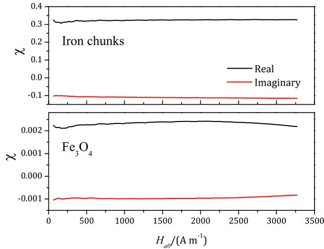
**Figure 8.** Susceptibility for iron chunks (top) and magnetite nanoparticles (bottom) both at 300 K.
