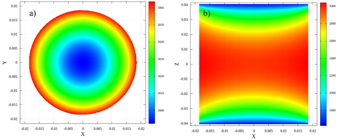
**Figure 4.**  $H_z$  component of the magnetic field for the driving coil. a) Plane  $x - y$  with  $z = 0$  and b) Plane  $x - z$  with  $y = 0$ . The colour scale is given in A/m and the coordinate axes are in m.
