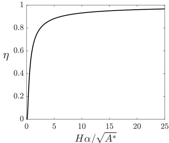
Figure 3: Emptying-filling box in steady state: Mixing efficiency  $\eta$ , as a function of the opening area  $A^*$ , box height  $H$ , and entrainment coefficient  $\alpha$ .
