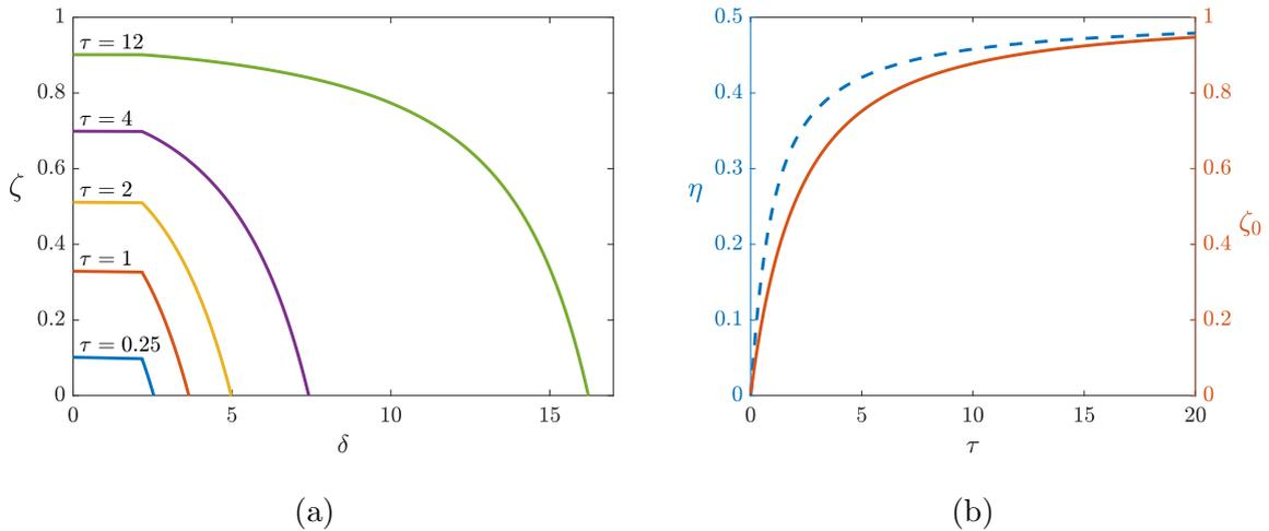
Figure 2: Filling box: (a) Dimensionless density profile at  $\tau = 0.25, 1, 2, 4, 12$ , (b) mixing efficiency  $\eta$  (blue, dashed) and the height of the mixed layer  $\zeta_0$  (orange, solid) against time non-dimensionalised by a filling box time scale, as defined in Eq. 6.
