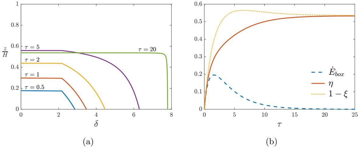
Figure 4: Emptying-filling box for  $A^* C^{-3/2} H^{-2} = 0.02$ : (a) Dimensionless density profile in an emptying-filling box at  $\tau = 0.5, 1, 2, 5, 20$ , (b) mixing efficiency of an emptying-filling box  $\eta$  (solid, orange), normalised rate of change of potential energy inside the box  $\dot{E}_{box}$  (dashed, blue) and the height of the mixed layer  $1 - \xi$  (dotted, yellow) against non-dimensional time.
