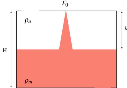
Figure 1: Steady state of the emptying-filling box with a point source of pure buoyancy (whose specific buoyancy flux is  $F_0$ ).  $H$  is the vertical separation between the openings,  $h$  is the distance from the upper opening to the interface. The buoyant mixed layer and ambient densities are labelled  $\rho_m$  and  $\rho_a$  respectively.
