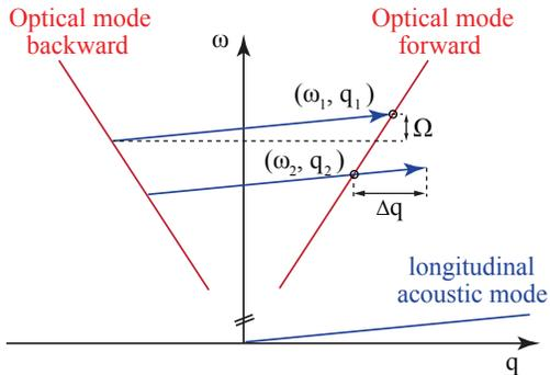
FIG. 3. Dispersion relation for the backward Brillouin scattering process at two different optical wavelengths.
