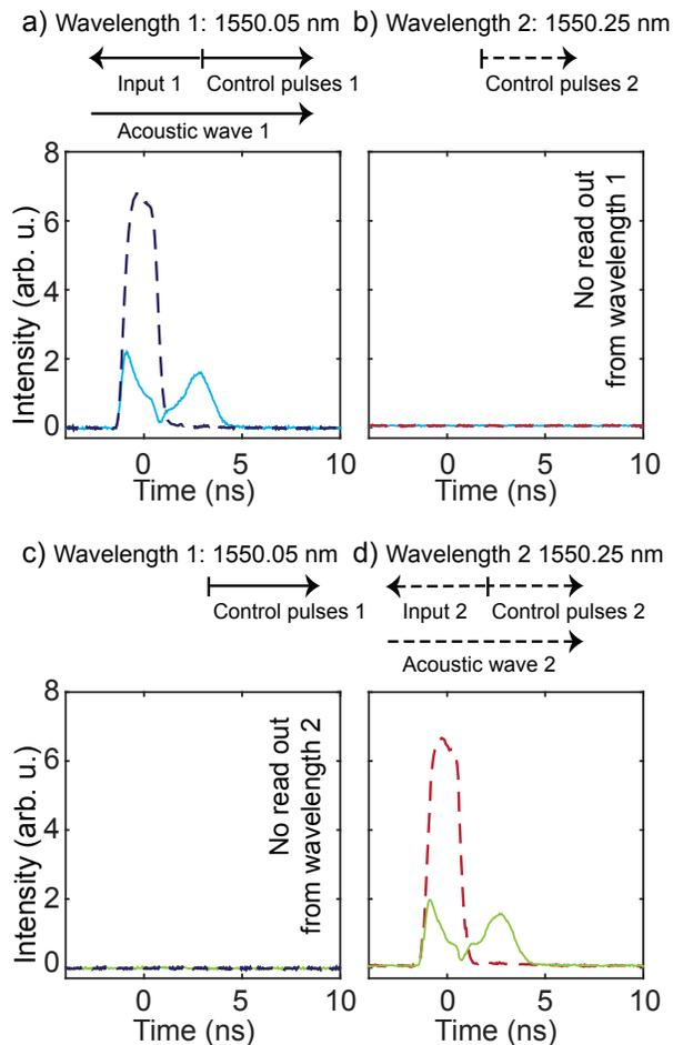
FIG. 6. a) The coherent transfer to the acoustic domain and back is operating at wavelength 1; b) no read-out is observed at wavelength 2 (light blue solid line); the dashed line represents the reference noise level of the photo diode as comparison. c) and d) The coherent transfer at wavelength 2 is operating while no read-out is observed at wavelength 1 (green line); the dark blue dashed line is the reference noise level of the photodiode.
