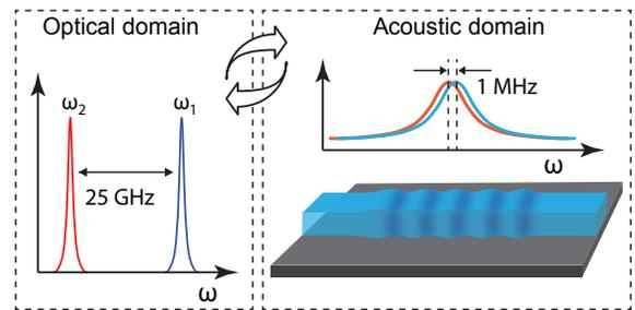
FIG. 1. Coherent transfer between the optical and acoustic domain. The two optical wavelengths are separated by  $2\pi\Delta F$ , here about 25 GHz. They are converted to two acoustic phonons which are separated by about 1 MHz, which lays well within the Brillouin linewidth.
