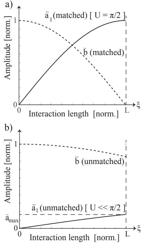
FIG. 11. Amplitude of the transfer of the acoustic phonon to the data pulse for the case of a) phase-matched pulses (same wavelength channel), b) phase-mismatched pulse (other wavelength channel).
