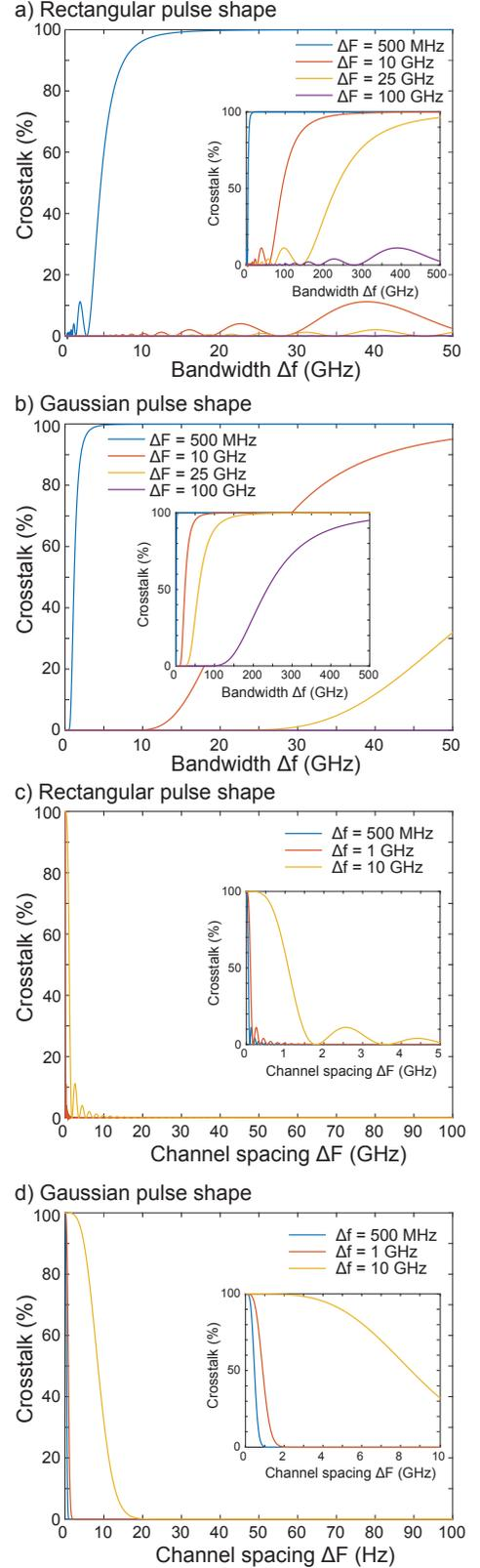
FIG. 12. Crosstalk study: a) and b) Fixed channel spacing  $\Delta F$  for varying bandwidth  $\Delta f$ ; c) and d) fixed bandwidth  $\Delta f$  and varying channel spacing  $\Delta F$ . The pulse shape is rectangular in a) and c) and Gaussian in b) and d). The respective insets zoom in or out of the x-axis with reasonable bandwidth and channel spacing for the purpose of demonstrating the behaviour of the crosstalk outside these practical values.
