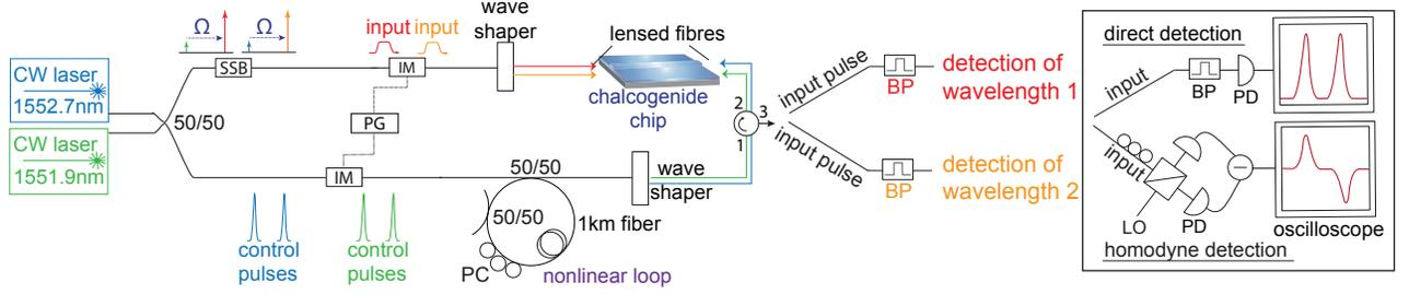
FIG. 4. Experimental setup for studying the coherent multi-wavelength Brillouin interaction: PC polarization controller, SSB single-sideband modulator, IM intensity modulator, PG pulse generator, BP bandpass filter, LO local oscillator, PD photo diode.
