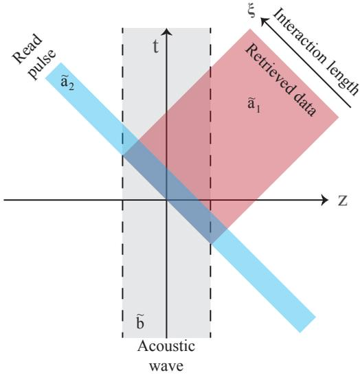
FIG. 10. Conversion of the acoustic phonon to a retrieved data pulse via the read pulse in the reference frame of the acoustic wave.
