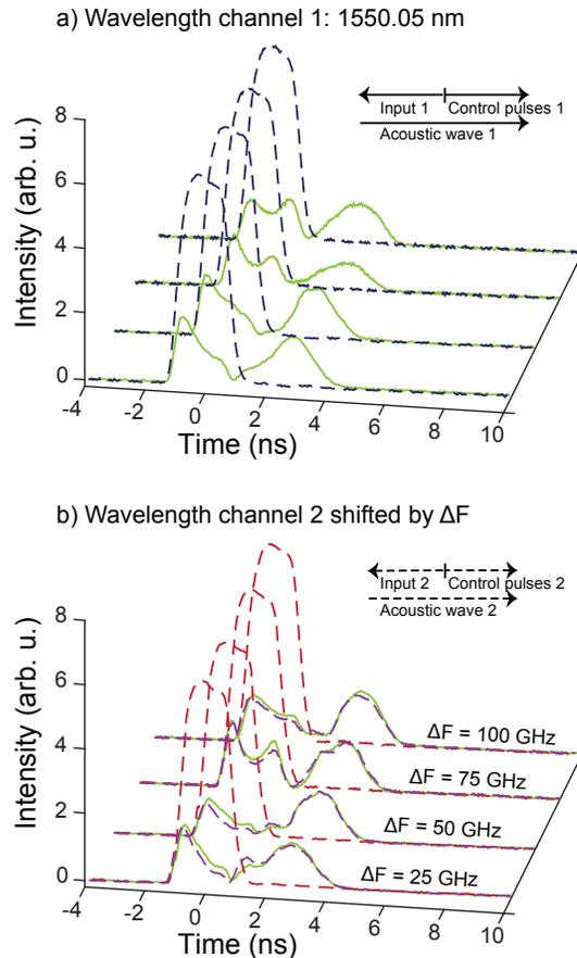
FIG. 8. Simultaneous storage at two wavelength channels for different frequency spacing of the two channels: 25 GHz, 50 GHz, 75 GHz and 100 GHz. The dashed lines correspond to the undepleted data pulses and the solid lines to the depleted and retrieved data. a) Wavelength channel 1. b) Wavelength channel 2. The violet solid line corresponds to single-channel storage at wavelength channel 2 only as a comparison to parallel storage operation at both wavelengths.
