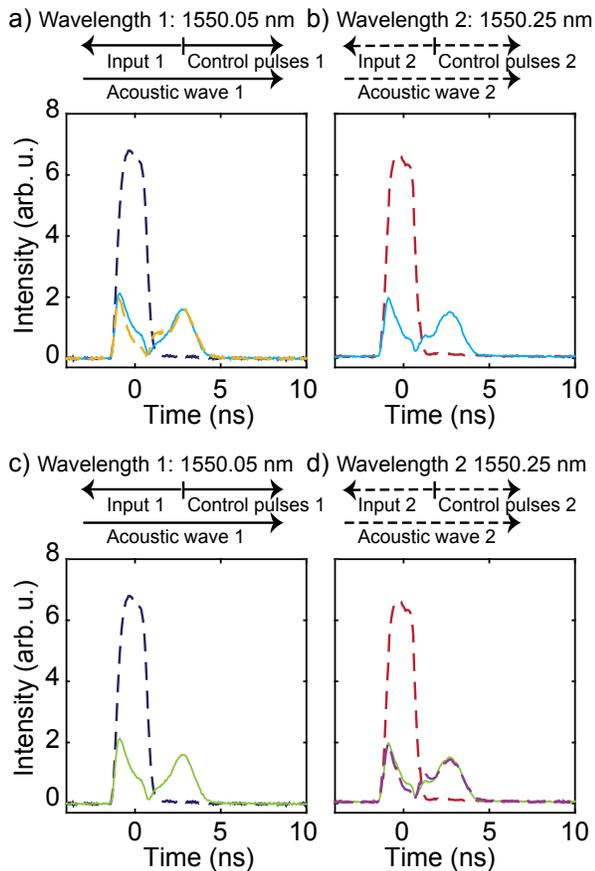
FIG. 7. a) and b) Simultaneous operation of the coherent transfer at wavelength 1 and 2. The dashed lines represent the original data pulses. The original data pulses are depleted and retrieved after 3 ns at both wavelengths (solid lines). The yellow graph in a) refers to a coherent transfer at wavelength 1 without memory operation at wavelength 2. c) and d) Comparison of simultaneous 2-channel storage operation to single-operation at wavelength 2 (violet solid line).
