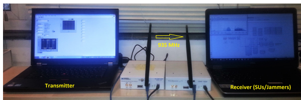
Fig. 7: Proposed USRP based experimental testbed.
