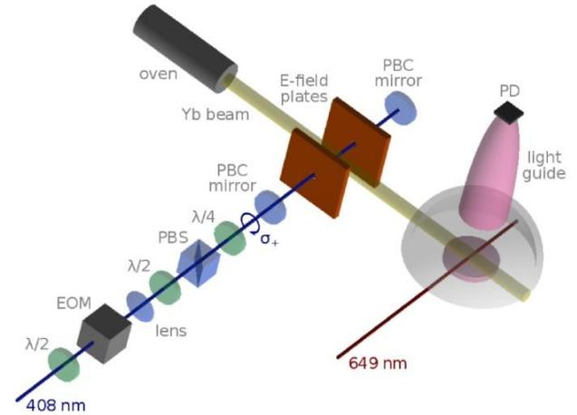
Fig. 2 (Color online). Schematic of the Yb atom-beam spectroscopy setup.  $\lambda/2$ : half-wave plate,  $\lambda/4$ : quarter-wave plate, PBS: polarizing beam-splitter, EOM: electro-optic modulator, PBC: power-build-up cavity, PD: photodiode.
