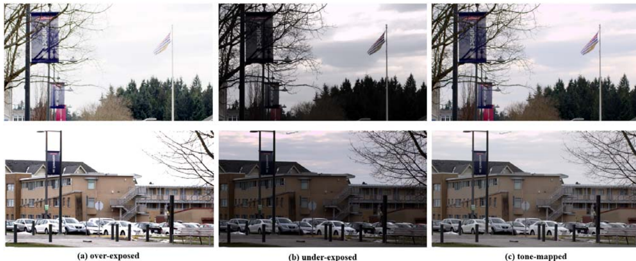
Fig. 4. Capturing with different exposure levels: (a) over-exposed, (b) under-exposed, and (c) tone-mapped. Note that tree colors are not visible in (b)-top, and airplane is not visible in (a)-bottom. Only right view frame is shown here.
