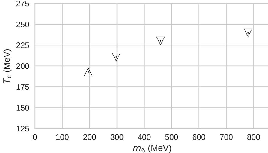
FIG. 4. Transition temperature  $T_c$  for the sextet-only theory with  $N_t = 6$  as a function of quark mass. The three heaviest ensembles (down arrows) are deconfined-side ensembles and thus give upper bounds on  $T_c$ . The lightest ensemble (up arrow) is a confined-side ensembles and thus gives a lower bound on  $T_c$ . The scale has been set via  $t_1 \equiv 1/(780 \text{ MeV})^2$ .
