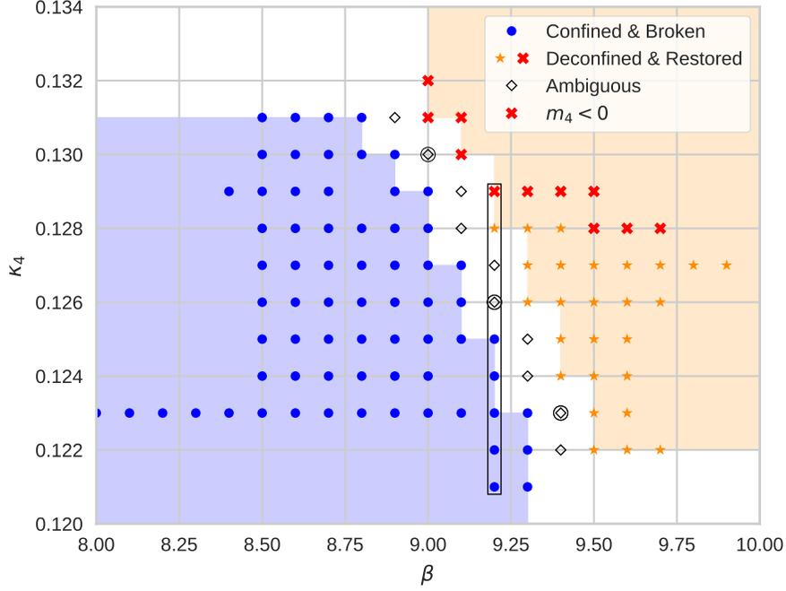
FIG. 6. Phase diagram for the fundamental-only limit on  $12^3 \times 6$ . Symbols and colors are as in Fig. 3, with the addition of hollow diamonds indicating ensembles in the crossover region, where the diagnostics are ambiguous. The black box indicates the slice through bare parameter space shown in Fig. 5. The circled ensembles have matching zero-temperature ensembles available.
