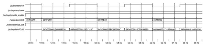
Fig. 5. Inputs and Output of Pan-Tomkin FPGA model in modelsim using co-simulation.
