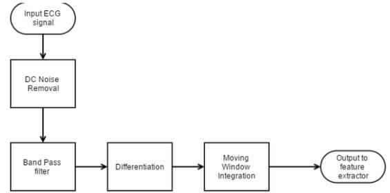
Fig. 2. Flow of QRS detection algorithm
