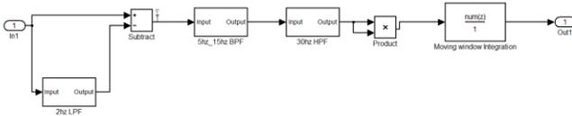
Fig. 3. Simulink model of QRS detector
