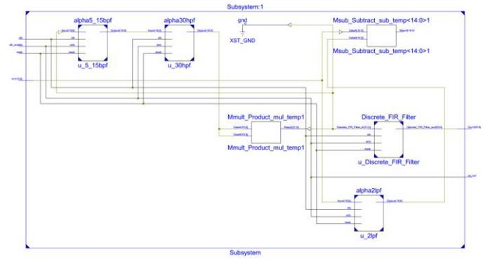
Fig. 4. RTL schematic of QRS detector
