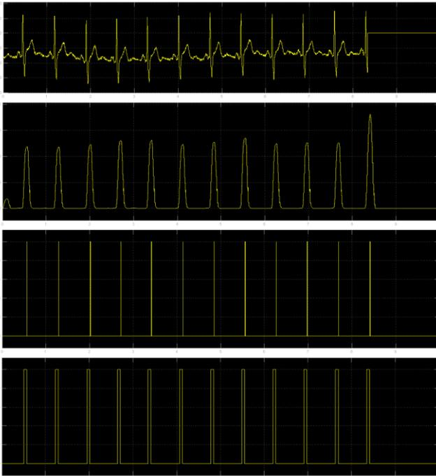
Fig. 6. Application of proposed algorithm to ECG signal. Row 1: ECG signal. Row 2: Output of Pan-Tomkin algorithm. Row 3: Extracted R-peaks. Row 4: Extracted QRS Interval.
