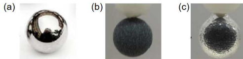
FIGURE 3. Images taken during the manufacturing procedure of a d = 10 mm SH sphere illustrating: (a) reference stainless steel sphere, (b) intermediate layer made of a carbon-based powder, (c) air plastron around the surface of the SH sphere once immersed in water.
