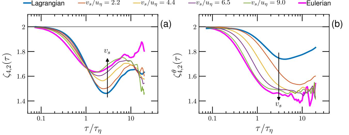
FIG. 7. (a) ESS local slopes, *i.e.*, logarithmic derivative of the fourth order moments of probe velocity time increments versus the second order one as in eq. (13). (b) Same as before for scalar increments. Remark the opposite intermittency trends between the velocity and the scalar at increasing  $v_s$  intensity (arrow direction).
