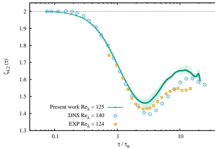
FIG. S1. Logarithmic derivative of the fourth order moments of Lagrangian fluid velocity time increments versus the second order one as in Eq. (13) of the paper. Comparison of present simulations at  $Re_\lambda = 125$  with simulations and experiments at comparable Reynolds number from Ref. [3].
