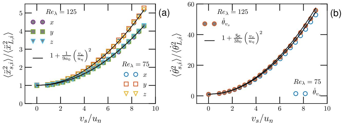
FIG. 2. a) Variance of the probe acceleration,  $\ddot{x}_{s,i}$  with index  $i$  denoting a Cartesian component, normalized by the variance of the fluid acceleration  $\ddot{x}_{L,i}$  as a function of the propulsion velocity  $v_s$ . The continuous line corresponds to the prediction (5). b) Variance of passive scalar time-derivative and comparison with the prediction (6).
