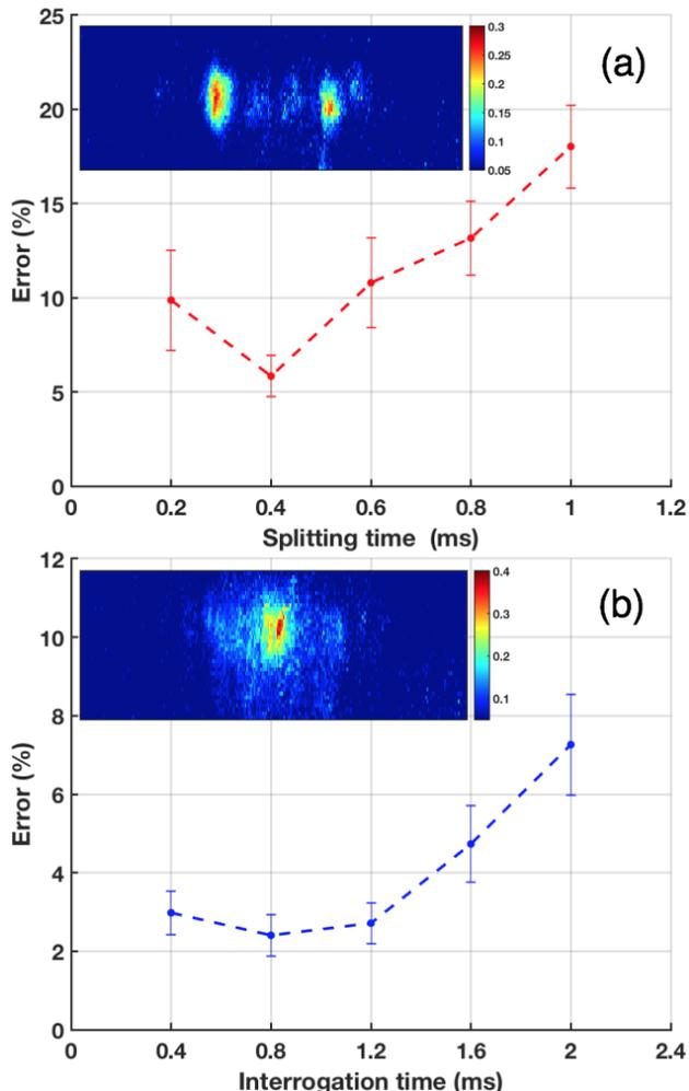
FIG. 3. Percent error in the (a) splitting and (b) recombination protocols as a function of (a) the splitting time  $T_1/2$  and (b) the total interrogation time  $T_1$ . (a, inset) An image from optimized splitting of the atoms into equal population in the  $\pm 2\hbar k_L$  momentum states and (b, inset) recombining the atoms into the ground Bloch state. The colorbar represents optical density (OD).
