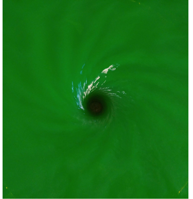
FIG. 3. Example of the spirals that can be observed close to the drain of a perturbed DBT vortex. Like the dominant mode we observe in our MOL simulations the spiral is counter propagating, hinting that resonant frequencies could provide a good description of this phenomenon. This image is taken from a vortex flow obtained using the experimental setup [34]. Here the water height is 5cm at the outer boundaries of the basin and the water is drained at a rate of 30 l/min through a hole of 4cm diameter. Although the presented flow is too deep to be accurately described by the two-dimensional equations (as in the text), we believe that the observed spiral is qualitatively similar to those studied in this paper.
