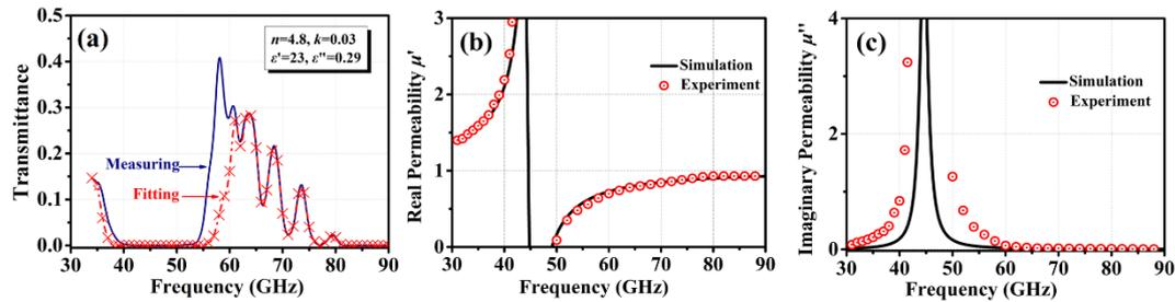
**Fig.4** Millimeter wave transmittance spectra, and real and imaginary parts of magnetic permeability in
