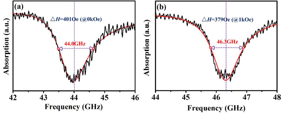
**Fig.3** The dependence of the frequency response of the resonance absorption in a crystallographically textured  $\text{Ba}_{0.8}\text{La}_{0.2}\text{Fe}_{11.8}\text{Cu}_{0.2}\text{O}_{19}$  sample: (a) at 0Oe; (b) at 1kOe.
