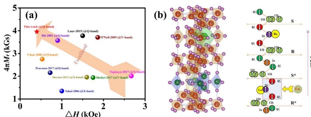
**Fig.1** Published values for remanent magnetization  $4\pi M_r$  and FMR linewidth  $\Delta H$  in bulk BaM and the corresponding crystalline structure of La-Cu substituted barium hexaferrites in this work
