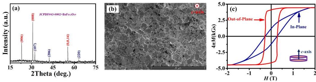
**Fig.2** The crystallographic, microstructural and magnetic properties of textured hexaferrites.
