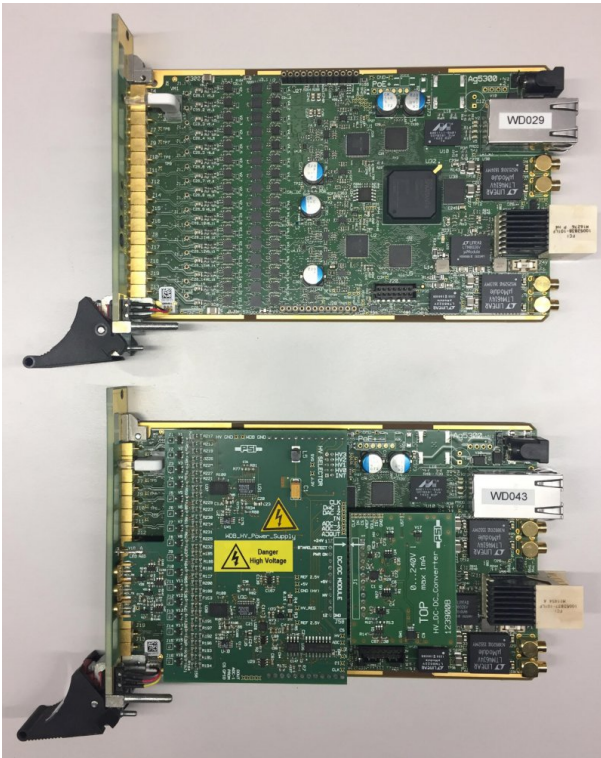
Figure 90 Two WaveDREAM boards without (top) and with a high-voltage piggy-back board (bottom).
