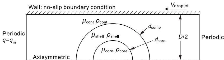
FIG. 1. Schematic configuration of the numerical simulation of a compound droplet in an axisymmetric microchannel.
