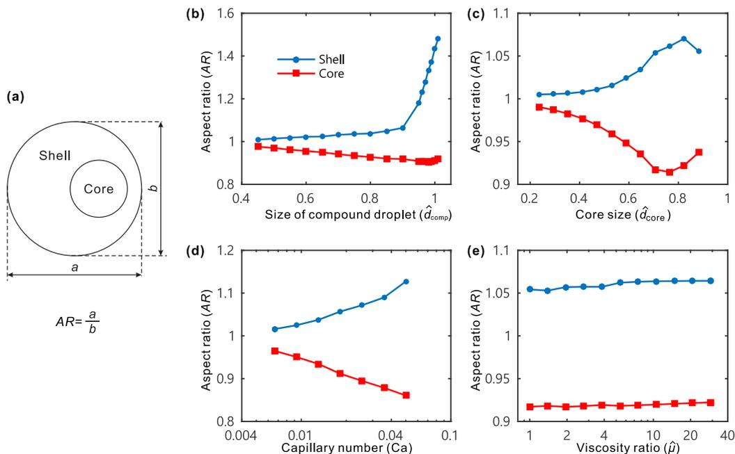
FIG. 8. Aspect ratio of compound droplets. (a) The aspect ratio is defined as the ratio between the length of the droplet in the flow direction and that in the spanwise direction, i.e.,  $AR \equiv a/b$ . (b) Effect of the size of compound droplets; (c) Effect of the core size; (d) Effect of the capillary number; (e) Effect of the viscosity ratio. The parameters are the same to those in FIG. 7.
