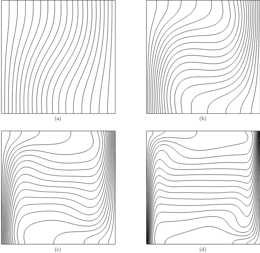
Figure 5: Isotherms of natural convection in a square cavity at: (a)  $Ra = 10^3$ , (b)  $Ra = 10^4$ , (c)  $Ra = 10^5$ , and (d)  $Ra = 10^6$ .
