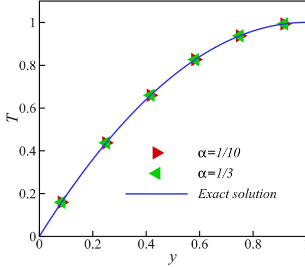
Figure 1: Comparison of temperature profiles predicted by the D2Q5 CLBM simulation and the analytical solution.
