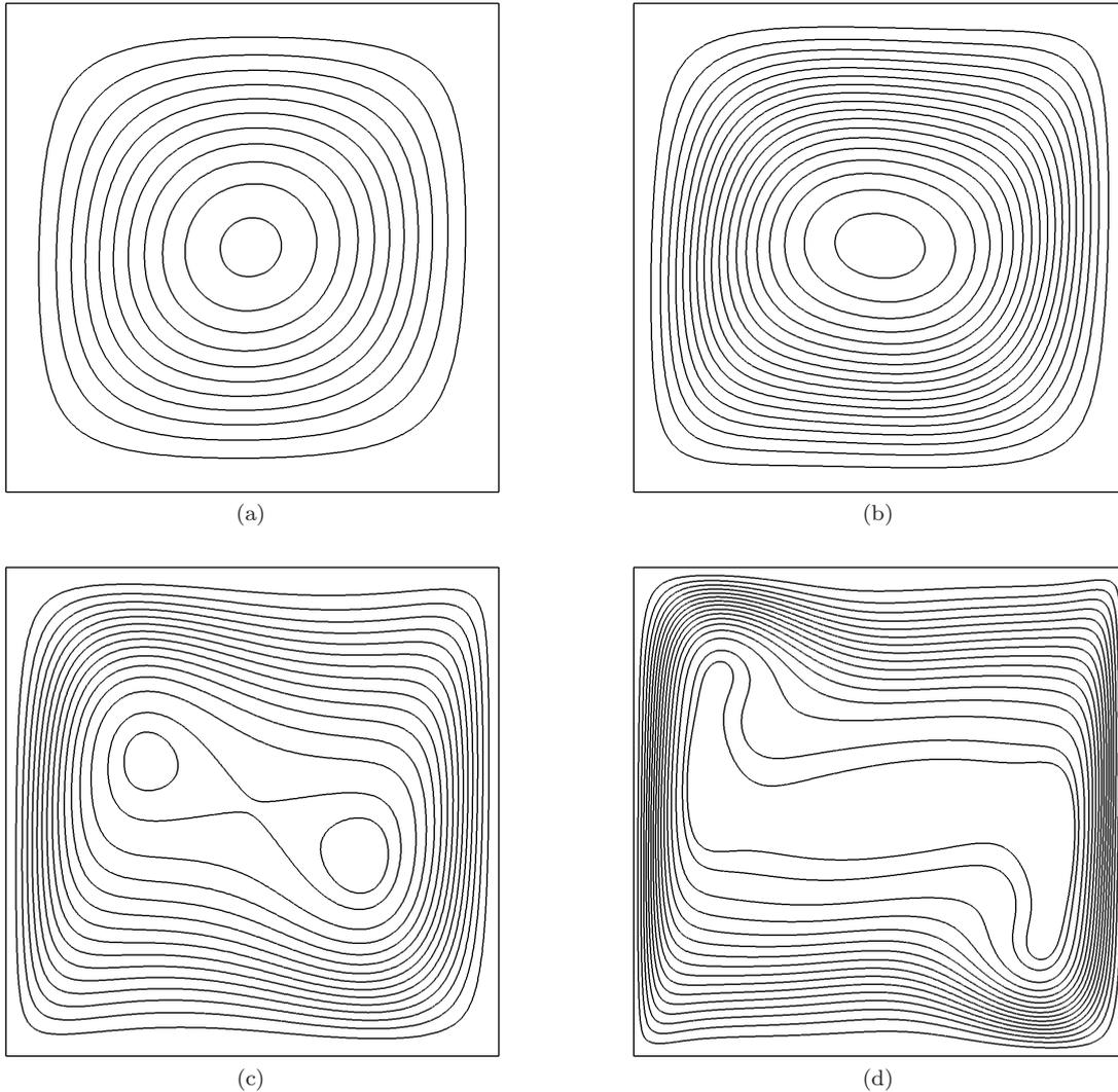
Figure 6: Streamlines of natural convection in a square cavity at: (a)  $Ra = 10^3$ , (b)  $Ra = 10^4$ , (c)  $Ra = 10^5$ , and (d)  $Ra = 10^6$ .
