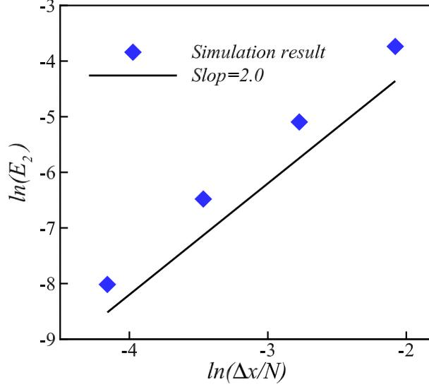
Figure 4: Global relative errors  $E_2$  change with grid sizes for viscous dissipation problem in Poiseuille flow.
