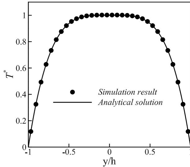
Figure 3: Comparison of the dimensionless temperature profiles predicted by the D2Q5 CLBM simulation and the analytical solution.
