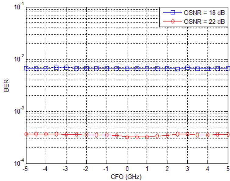
Fig. 8. BER vs. CFO for 800-km SSMF transmission.
