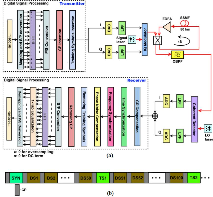
Fig. 1. (a) Simulation setup of the RGI-CO-OFDM system. (b) OFDM frame structure. S/P: serial-to-parallel conversion. P/S: parallel-to-serial conversion. LPF: low-pass filter. OBPF: optical band-pass filter. SYN: synchronization symbol. DS: data symbol. TS: training symbol.
