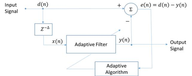
Fig. 2. Block diagram representation of feedback ANC system
