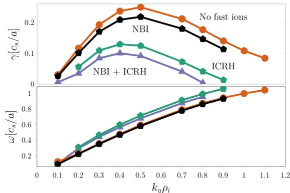
**Figure 2.** ITG growth rate and frequency spectra with different concentrations and types of fast ions. Orange circles show the case without any fast ions (case B<sub>Xe</sub> of Table A2), black/green pentagons show a case with only the NBI/ICRH fast ions with  $Z_f n_f = 0.06/0.14$  (cases B<sub>N</sub>/B<sub>I</sub>, respectively), and violet triangles show the baseline case (B<sub>0</sub>) with both NBI ( $Z_f n_f = 0.06$ ) and ICRH ( $Z_f n_f = 0.14$ ).
