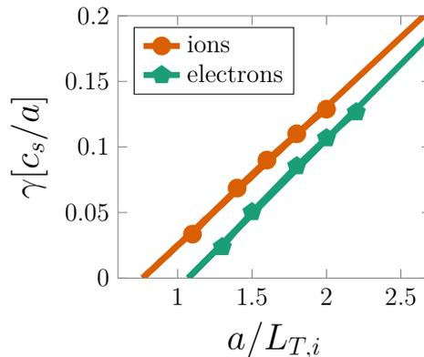
**Figure 3.** ITG mode growth rates at  $k_y \rho_i = 0.57$ , as a function of the driving temperature gradient. In one case, we assume that the thermal ions replace the removed fast ions (orange circles - case BXi of table A2). In the other, electrons are removed along with fast ions (green pentagons - case BXe).
