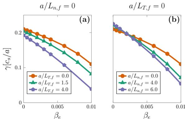
**Figure 6.** Scan of growth rate versus  $\beta_e$  for different fast ion species: (a) ICRH-like, and (b) NBI-like, each with several different gradients of temperature and density, respectively. These are iterations of cases BI0 and BN0 of Table A2 with the fast ion gradients adjusted as indicated. For Case BN0, electron density and density gradient are likewise adjusted to maintain quasineutrality.
