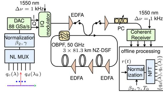
**Fig. 2:** Experimental setup with offline NFT-based detection
