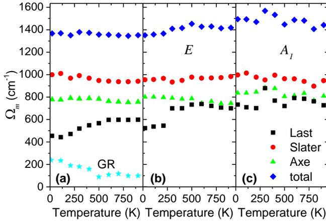
FIG. 14. Temperature dependence of the mode-plasma frequencies  $\Omega_m$  of the main modes and the total plasma-mode frequency (from (a) model (i) and (b, c) model (iv)). GR stays for the geometrical resonance.
