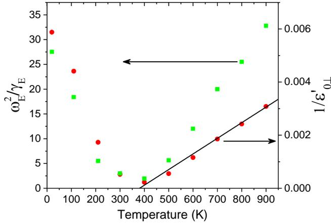
FIG. 16. Temperature dependence of the reciprocal static permittivity  $1/\epsilon'_{0\perp}$  (full circles) from Fig. 10 fitted with the Curie-Weiss law  $\epsilon'_{0\perp} = C/(T-T_C)$  ( $C = 1.7 \times 10^5 \text{ K}$ ,  $T_C = 380 \text{ K}$ ) (full line) and compared with the temperature dependence of the overdamped  $E$ -component of the SM characterized by  $\omega_E^2/\gamma_E$  – full squares.
