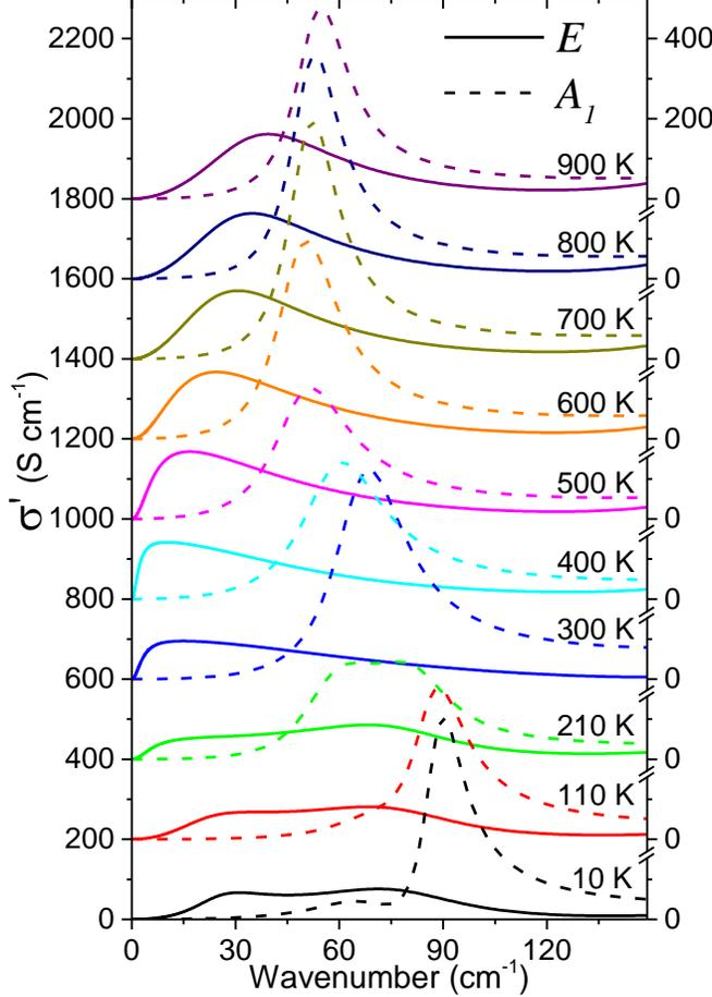
FIG. 11. Temperature dependence of the conductivity spectra for the SM components of the  $A_1$  (dashed) and  $E$  response (full lines) from model (iv). Each spectrum at the corresponding temperature is shifted by  $200 \text{ S cm}^{-1}$  with respect to the previous temperature and the values on the left-hand y-axis match the spectra at  $10 \text{ K}$ , while on the right y-axis the proper scale is adapted for all the spectra.
