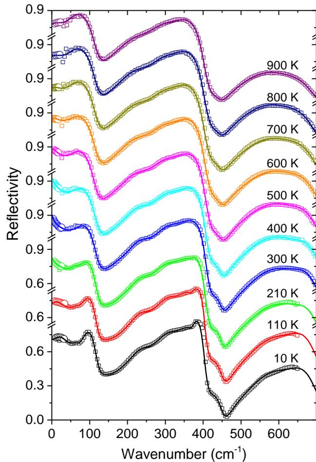
FIG. 1. Measured unpolarized IR reflectivities (squares) of the PMN crystal together with the calculated THz data (circles) and the factorized formula fits using the Eqs. 1 and 2 (full lines) in the 10–900 K range (model (i)). The fitted reflectivities agree with the data within the limits of experimental accuracy.
