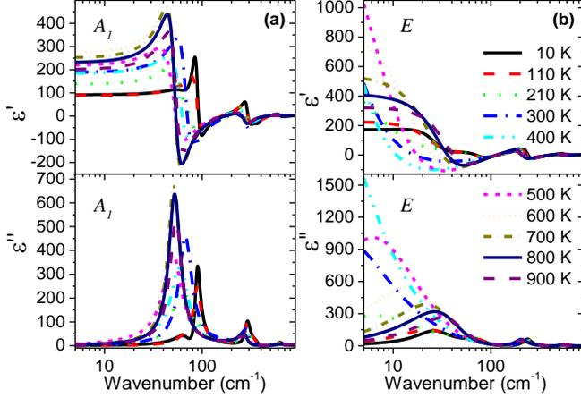
FIG. 9. Complex dielectric spectra of (a)  $A_1$  ( $\mathbf{E} \parallel \mathbf{P}_j$ ) and (b)  $E$  ( $\mathbf{E} \perp \mathbf{P}_j$ ) symmetry as evaluated from the fits in Figs. 7 and 8 (model (iv)) at selected temperatures (log-wavenumber scale).
