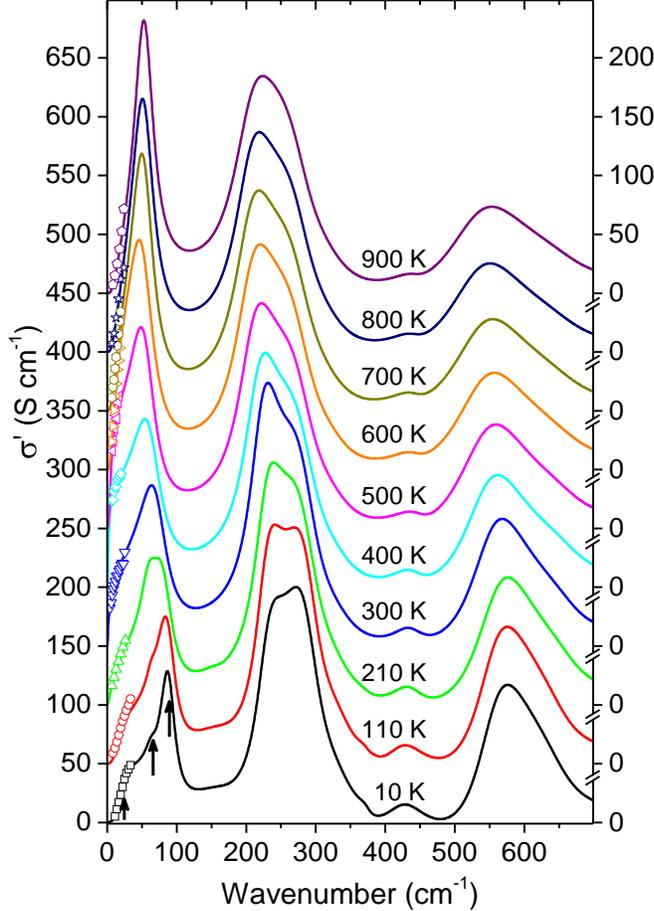
FIG. 3. IR conductivity spectra (full lines) calculated from the fits in Fig. 1 (model (i)), including the THz data (symbols). Each spectrum is shifted by  $50 \text{ S cm}^{-1}$  with respect to the previous one and the values on the left-hand y axis match the spectrum at 10 K, while on the right-hand y-axis the proper scale is adapted for all the spectra. Arrows mark the three SM features analyzed below (see Fig. 6).
