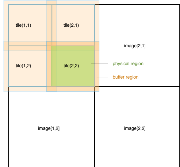
FIG. 2.— Spatial decomposition in CUBE in a 2D analogy. In this example, there are two images per dimension ( M_g = 2 ), and two tiles per image per dimension ( M_t = 2 ). The orange boxes show the overlapped extended ( V_e ) = physical ( V_p ) \cup buffer ( V_b ) tile regions. One physical region is indicated in green.
