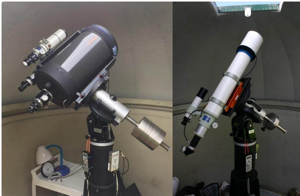
Figure 11: The author's observatory equipped with (a) 28 cm SCT and (b) 10 cm refractor
